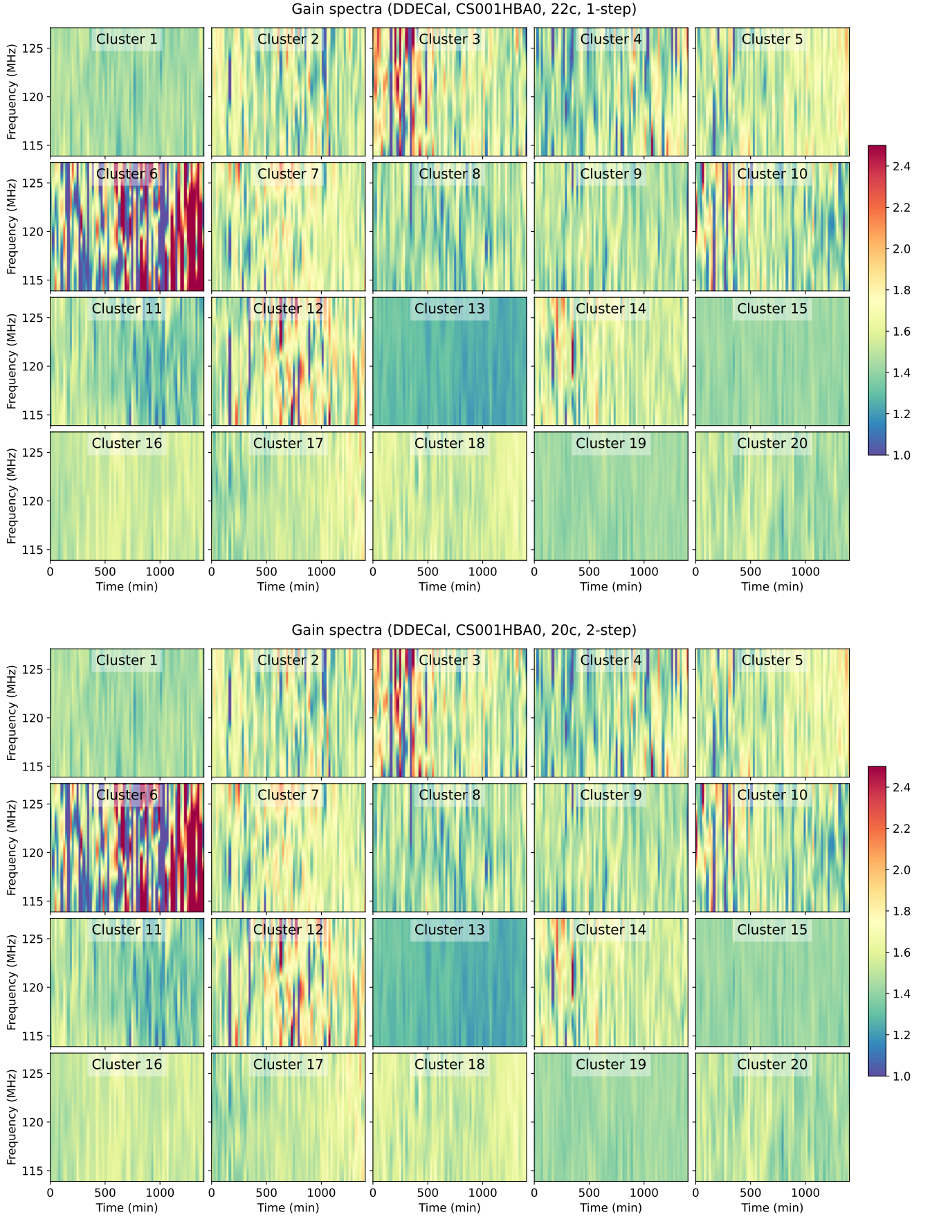
Fig. E.1. Gain dynamic spectra obtained by DDECAL algorithm for 20 clusters around the phase centre, using the one-step method (top) and two-step method (bottom) for one station (CS001HBA0). The different polarisation components are added in quadrature.
