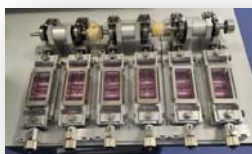
Figure 2. Custom-made uniaxial stretch machine.
