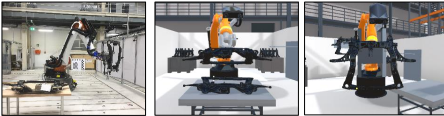
Figure 1. Real scenario (left), comparison of HRC-level 1 (middle) and HRC-level 3 (right). Pictures taken from participants' view in a virtual environment. In HRC-level 1, the robot moved to a waiting position after simulated placing of front axle carriers on the table (see middle).
