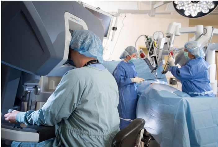
Figure 2. The da Vinci Surgical System includes a control console where the surgeon is seated (left) and surgical instrument dock that is positioned over the patient (right). Image from: https://www.franciscanhealth.org/health-care-services/robotic-assisted-surgery-334
