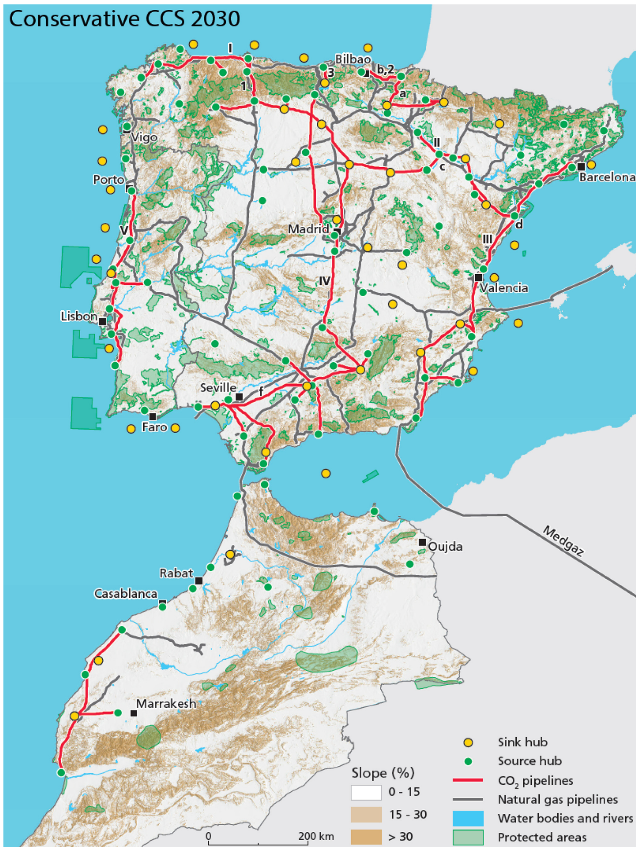
Fig. 2. CO 2 pipeline networks in the Conservative CCS scenario in 2030. The source and sink hubs represent the end points of the CO 2 pipelines. The geographical slopes, current natural gas pipelines, water bodies and protected areas are shown to illustrate potential interactions with the CO 2 pipelines. (For interpretation of the references to color in the text, the reader is referred to the web version of this article.)
