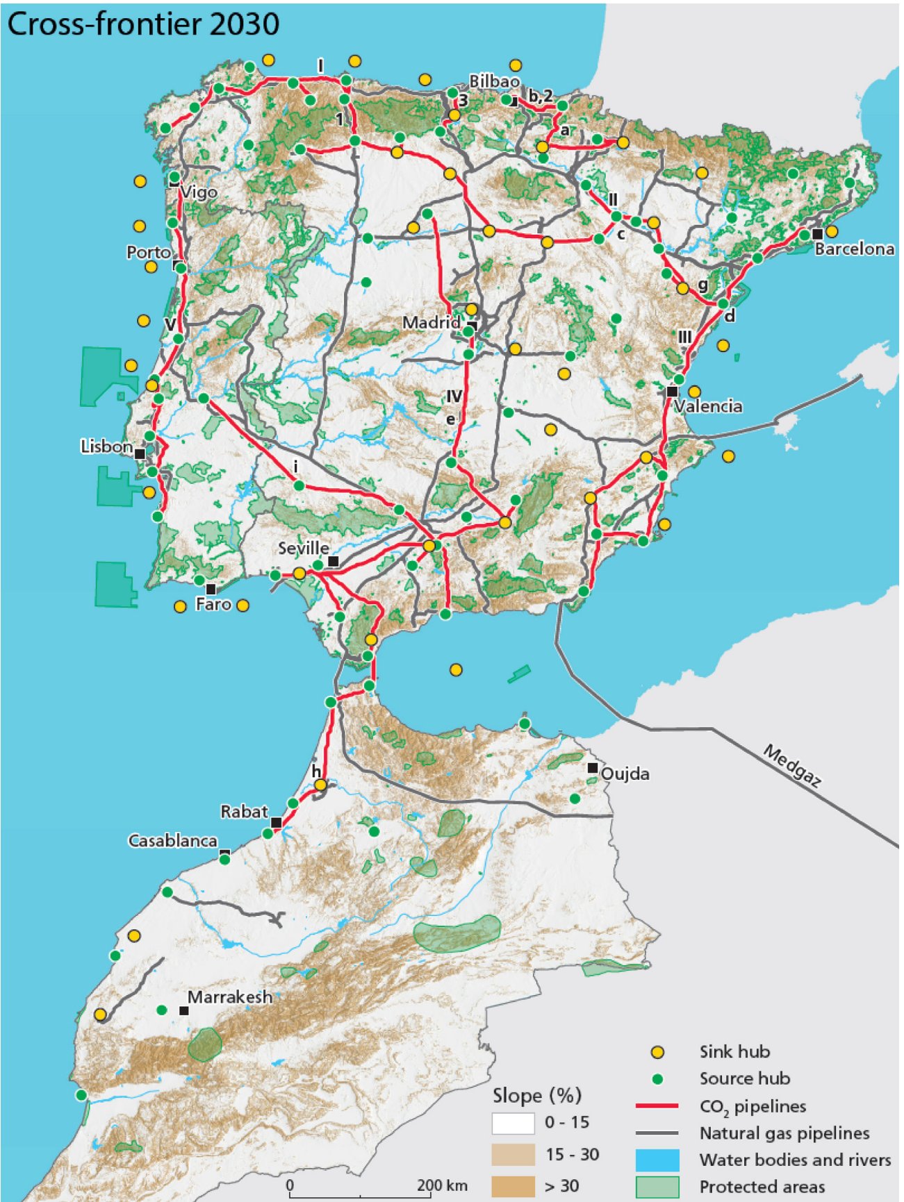
Fig. 3. CO 2 pipeline networks in the Cross-frontier scenario in 2030. The source and sink hubs represent the end points of the CO 2 pipelines. The geographical slopes, current natural gas pipelines, water bodies and protected areas are shown to illustrate potential interactions with the CO 2 pipelines. (For interpretation of the references to color in the text, the reader is referred to the web version of this article.)
