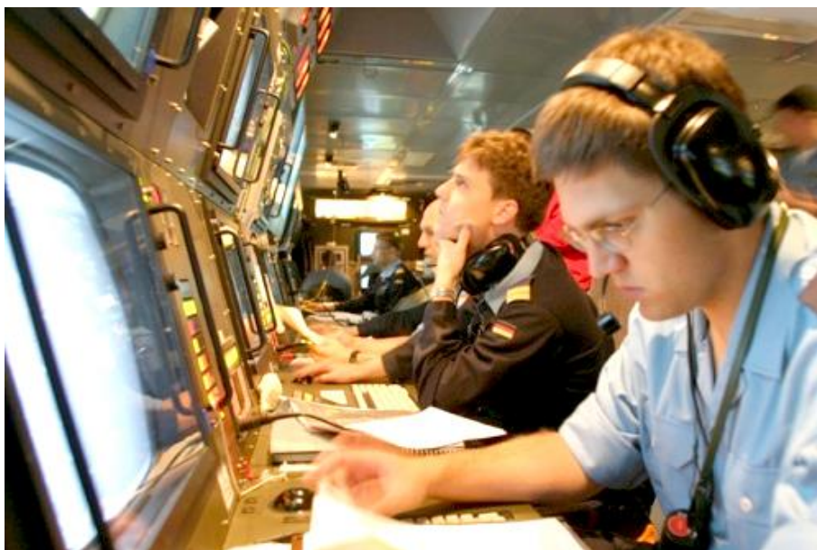
Figure 1. Typical workstations in a Combat Information Centre of a German frigate. Note the recessed trackball at the bottom of the picture. © Bundeswehr.
