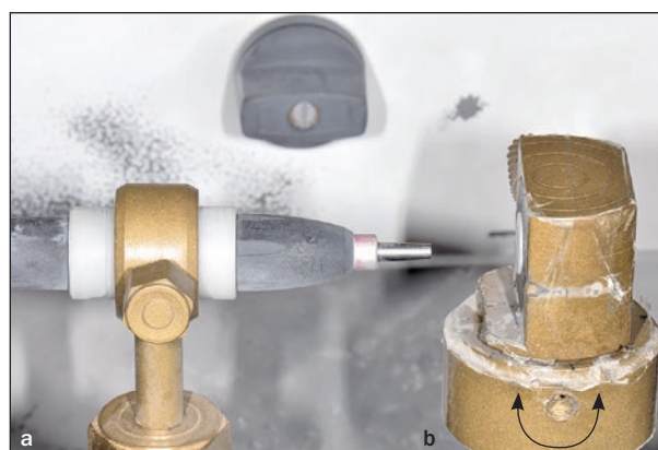
Fig 2 Adjustable device. (a) Jet tip is fixed. (b) Disk is positioned and can rotate 180 degrees.
