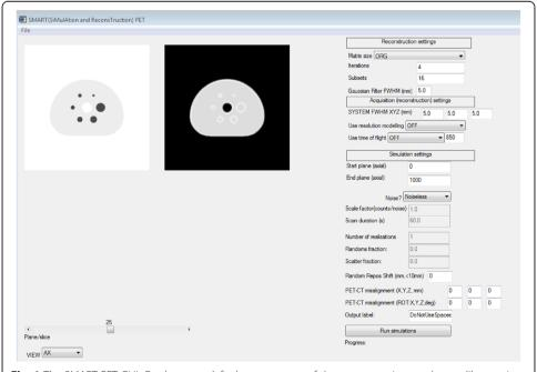
**Fig. 1** The SMART-PET GUI. On the upper left, the parameters of the reconstruction can be set, like matrix size, number iterations/subsets, resolution modelling ON/OFF and TOF ON/OFF. On the lower left, the simulation parameters like system sensitivity, random/scatter fractions and scan duration can be assigned
