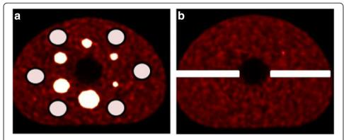
**Fig. 2** The regions of interest used to **a** calculate the COV in the phantom background at slice 38 and **b** the intensity distributions of the standard deviation image at slices 53–57 (right). Both images are generated using the physical phantom data, but the regions of interest are equally extracted from the corresponding slices of the simulated data
