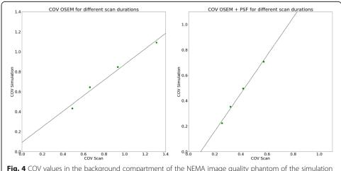
**Fig. 4** COV values in the background compartment of the NEMA image quality phantom of the simulation against the COV values of the scan for OSEM (left) and OSEM+PSF (right) reconstructions
