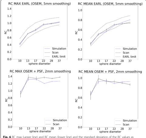
**Fig. 6** RC max (upper line) and RC mean (lower line) and the standard deviation of the RC values as function of sphere sizes for EARL reconstruction (OSEM + 5 mm smoothing) on the left and OSEM+PSF reconstruction with 2 mm smoothing on the right
