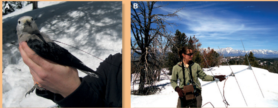
Fig. 12.B1.01 Radio-tracking devices for studying avian movements. (A) Researchers can attach small radio tags to a bird, here on the back feathers of a Clark's Nutcracker ( Nucifraga columbiana ), to monitor its movements. (B) Radio receivers and large antennas allow researchers to pinpoint a tagged bird's whereabouts after it is released back into the wild. (Photographs by Pocholo Martinez.)
