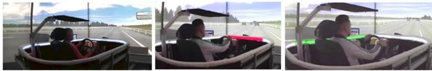
Figure 7. a) Ambient light active, b) Longitudinal warning, c) Lane change recommendation
