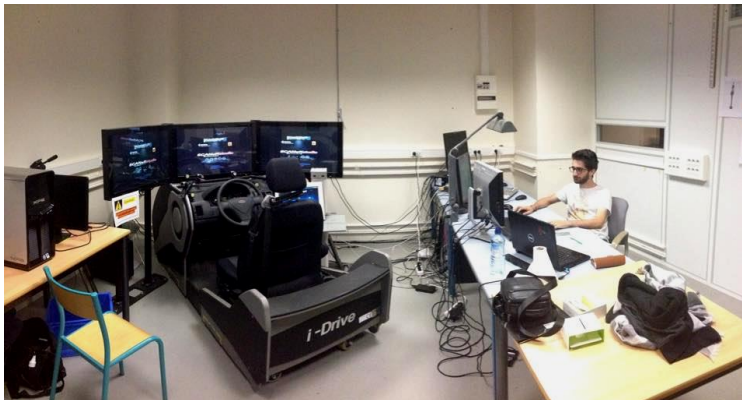
Figure 4. Picture of the fixed-base simulator used for the driving tests
