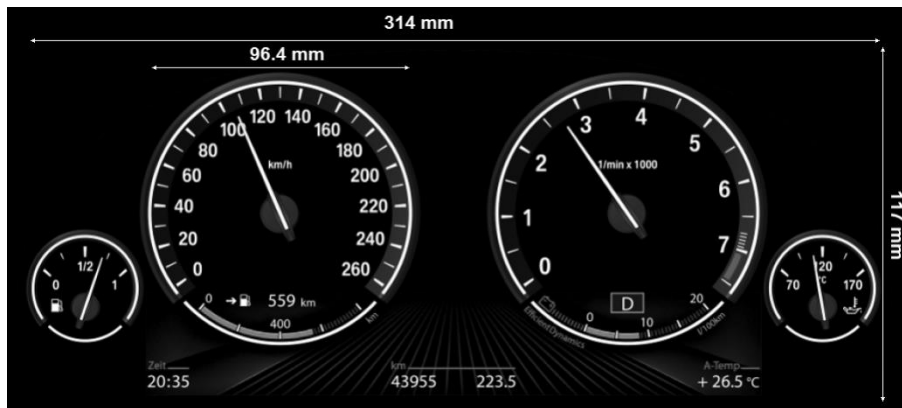
Figure 2. The cockpit concept used in this study with its measurements
