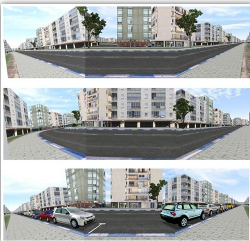
Figure 4. The Field of View factor as displayed in the virtual scenarios: (1) Unrestricted (above); (2) Partially obscured by the road's curvature (middle); (3) Partially obscured by parked vehicles (below).
