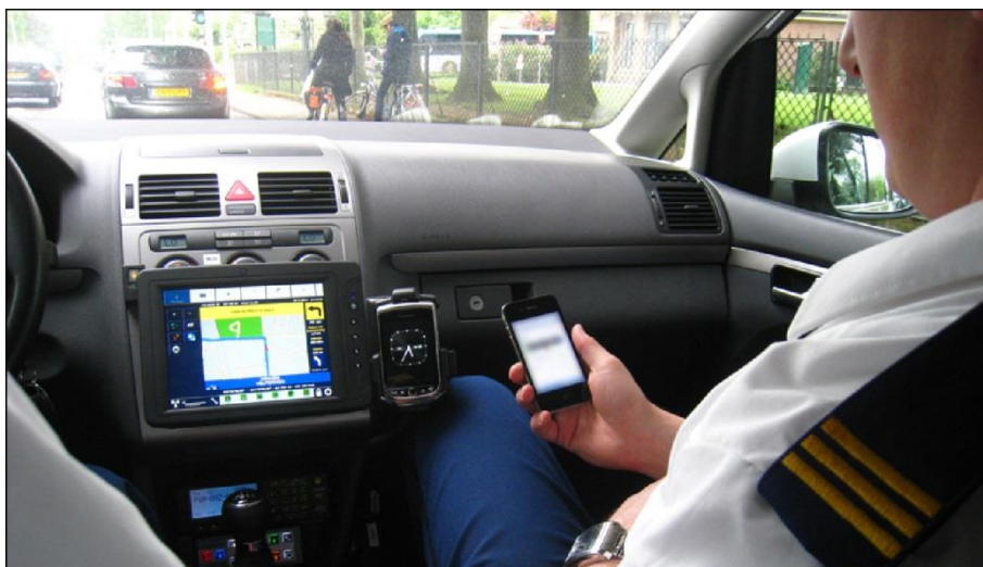
Figure 1. View on the cockpit of a police vehicle. The Mobile Data Terminal is located between the driver and co-driver.
