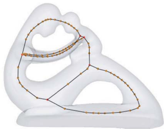
Fig. 1. Example an homotopic skeleton which has been produced by the 'Telea and Jalba' method. The skeleton is topologically equivalent to the original object which shown light grey in the background. Image from [3]
