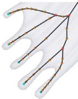
Fig. 5. Example of a detail preserving skeleton which has been produced by the 'Telea and Jalba' method. All details are captured well and the skeleton reaches into all toes of the frog foot. Image from [3]
