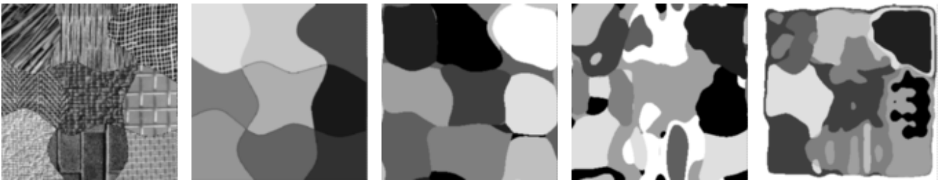
Figure 3. Results of segmentation experiments using the K-means clustering algorithm. The left-most image shows an input image containing nine different textures. The exact segmentation of the input image is shown in the second image from the left. The three right-most images show the segmentation results based on the grating cell operator features (middle column), the Gabor-energy features (second column from the right) and the cooccurrence matrix features (right-most column).
