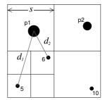
Figure 4: Space decomposition using quadtrees
