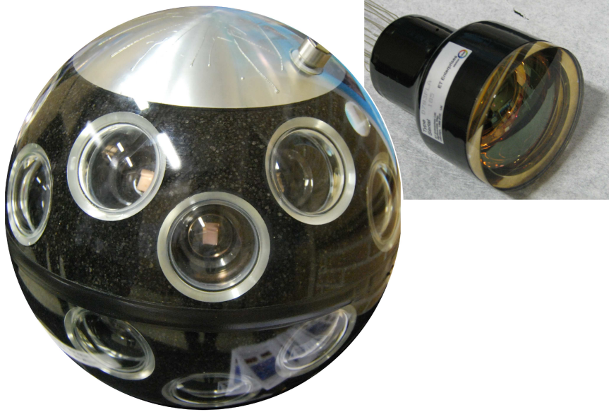
Figure 8.2: Prototype of the multi-PMT DOM with 31 3-inch PMTs arranged in a 17-inch diameter pressure glass sphere. Insert top right: the photograph of the ET Enterprises Ltd. D783FL 3-inch diameter PMT which was investigated by us and found suitable for KM3NeT [H + 12].
