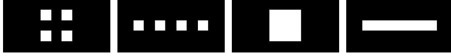
Figure 3.4: The elongation measures of the clustered sets X and Y (first and second image from the left) are similar if the we compute the C-attributes. The M-attributes instead are computed on \psi(X) and \psi(Y) (third and fourth image from the left respectively) and obviously the elongation of \psi(X) is smaller compared to that of \psi(Y) .
