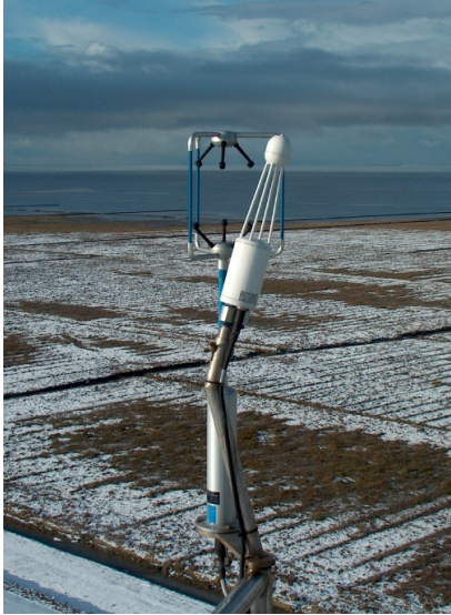
Fig. 2.7. Eddy covariance system at a height of 50 m.
