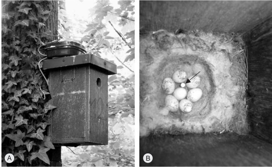
Picture 5.1. Nest box with box attached to it. Inside the box was the data logger that recorded incubation temperature. B) Great tit clutch with a sensor placed in between the eggs (see arrow).
