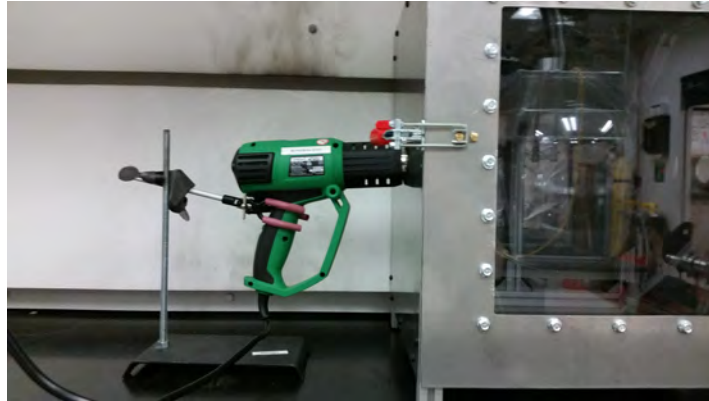
Figure 6.1: Heating System: Heat Gun.
