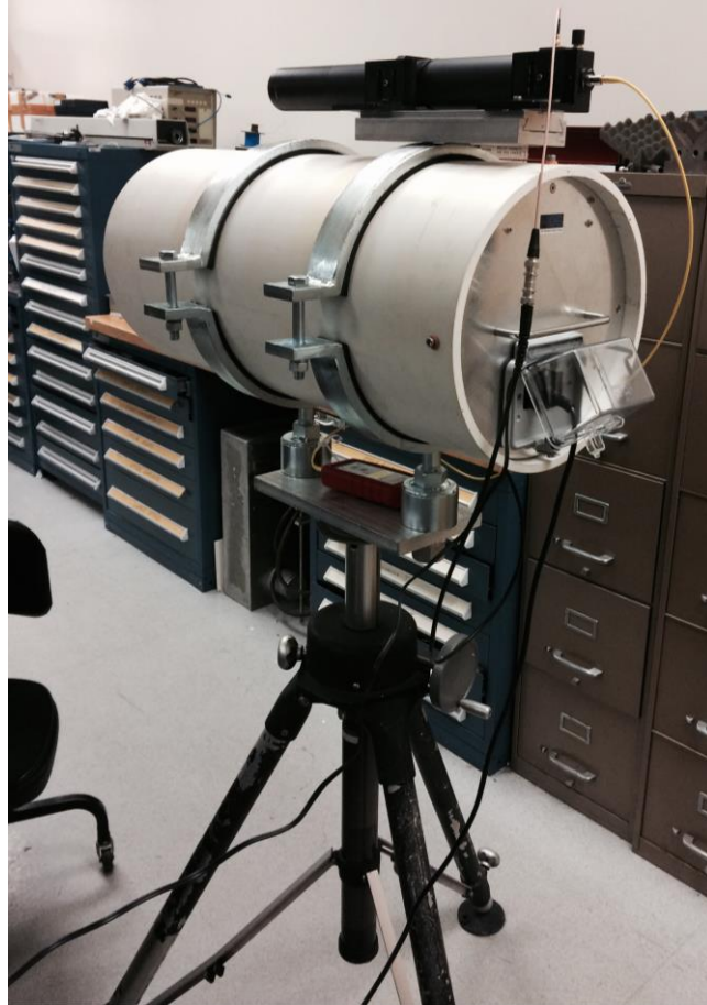
Figure 6. 9: Laser and LED integrated scintillometer's transmitter
