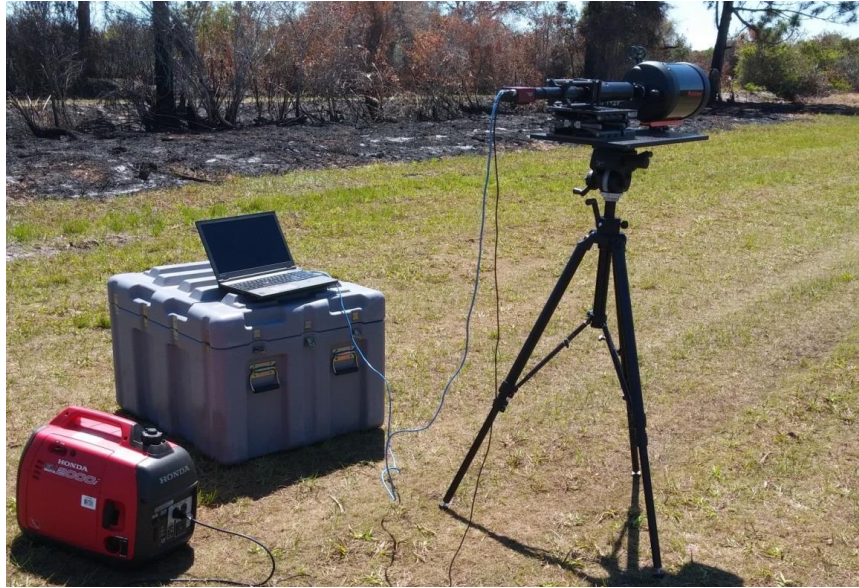
Figure 6. 39: Experimental picture of using the plenoptic sensor to observe scintillation index
