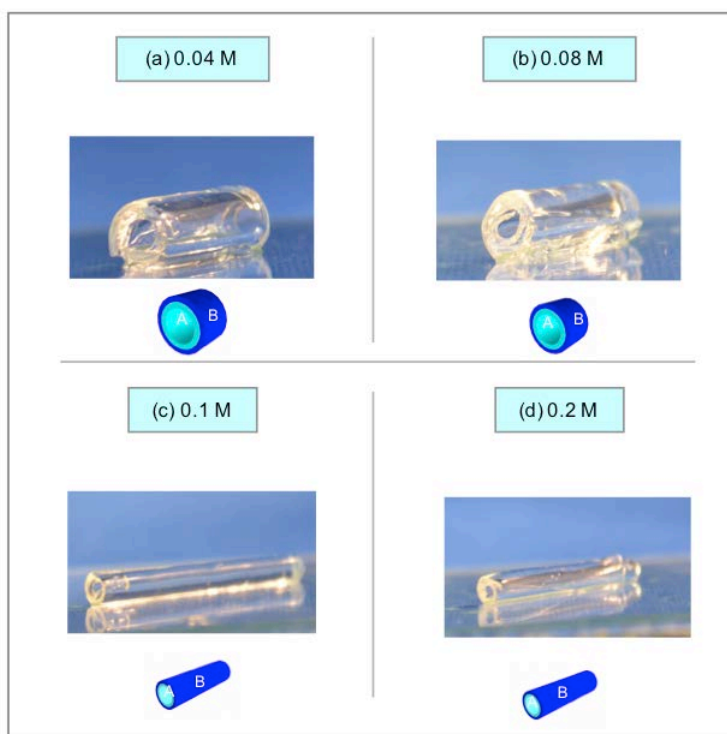
Figure 5.4. Effect of \text{Ca}^{2+} concentration on gel folding. The gels demonstrate short-side folding at low concentrations of \text{Ca}^{2+} and long-side folding for \text{Ca}^{2+} of 100 mM and above.
