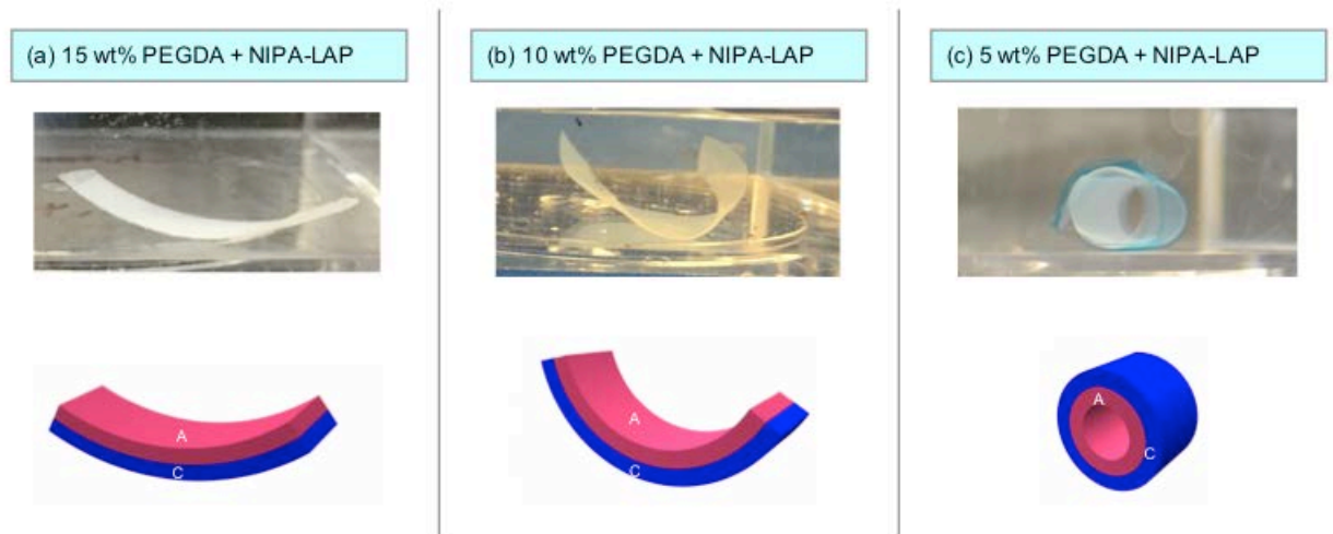
Figure 3.7. Folding behavior of bilayers of Gel A (PEGDA) and Gel C (NIPA-LAP). The dimensions of each gel was maintained at 20 mm x 9 mm x 0.15 mm. The NIPA-LAP is identical to that in Figures 3.3 to 3.6. The concentration of PEGDA was decreased from (a) to (c). Note that folding of the flat sheet into a tube is observed only when the PEGDA is reduced to 5 wt%. At higher concentrations of PEGDA, the stiffness of the A layer opposes folding.
