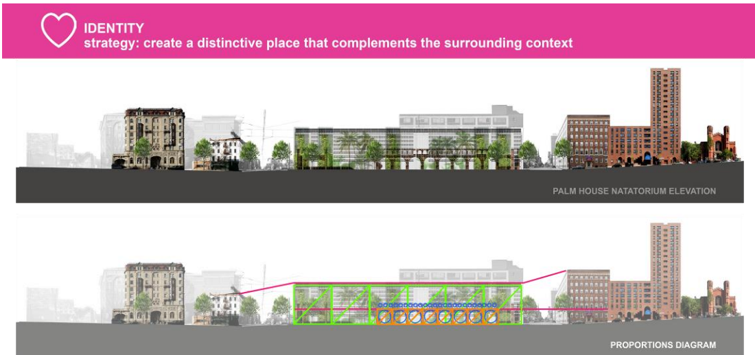
Figure 54 Elevation of the test building in context, showing contrast and distinction, material relationship, scale relationship, and building proportions.
