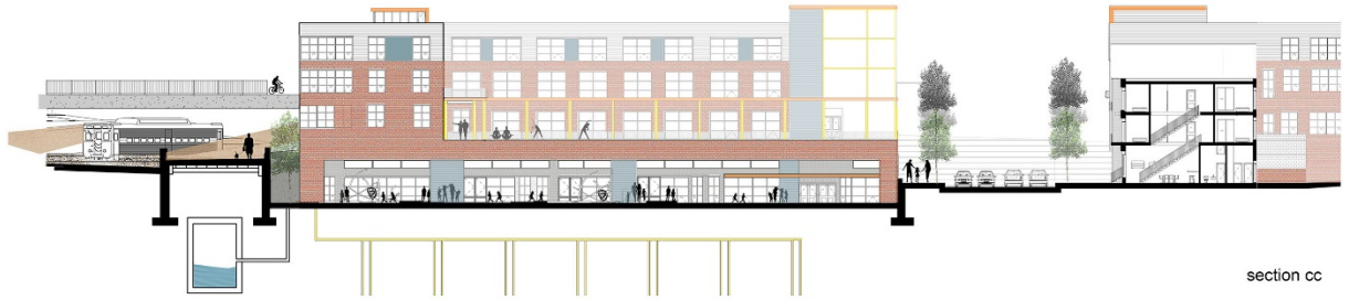
Figure 62: Proposed Section - through MARC ramp, Garden, Housing (Author)
