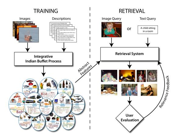
Figure 3.1: Schematic overview of our retrieval algorithm. The flow chart illustrates discovery of abstract features from multimodal data, the retrieval system for cross-view queries and user relevance feedback.
