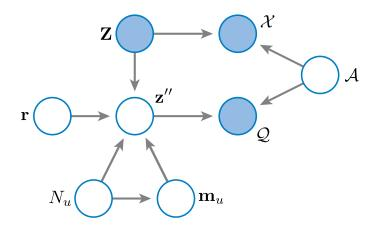
Figure 3.4: Graphical model for the feedback query model. Circles indicate random variables, shaded circles denote observed values. Hyperparameters are omitted for clarity. Note that  $\mathbf{Z}$  is considered as an observed variable in the retrieval part.
