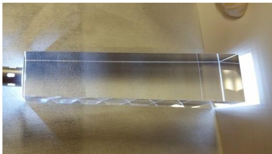
Figure 10: Demonstration of the internal reflections within the polished quartz light guide. Note how the diffuse light sourced on the left is redirected within the light guide and exits through the base located on the right.
