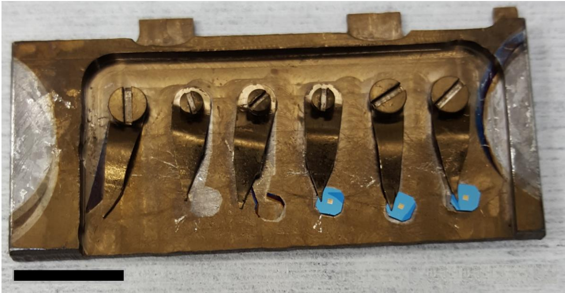
Figure 2.15 Sample holder. Optical photograph of SiN substrate samples clipped into deposition and milling holder. The frame is made from Al and the clips are Be/Cu. The holder is colored due to various materials depositions. Scale bar is 0.5 inches.
