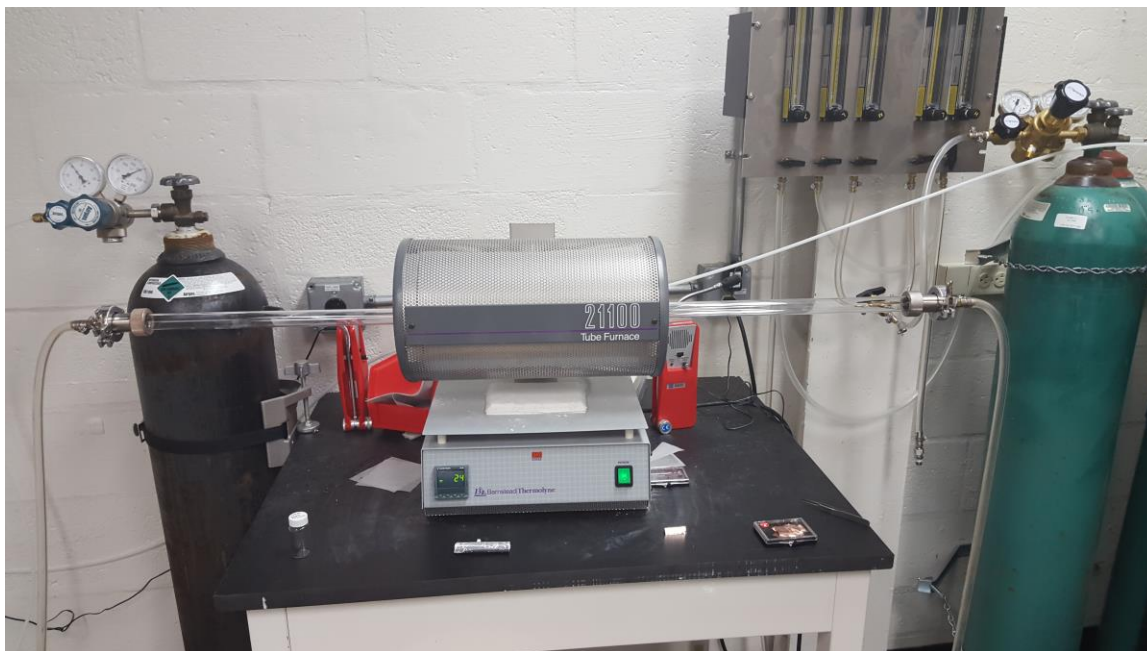
Figure 2.32 Tube furnace. The samples are inserted into the glass tube and positioned in the middle of the furnace. Ar gas flows from the cylinders on the right through the furnace to heat the samples without oxidizing them. To quench the samples, the glass tube can be quickly slid far to the right so that the samples leave the middle section where the heat source is.
