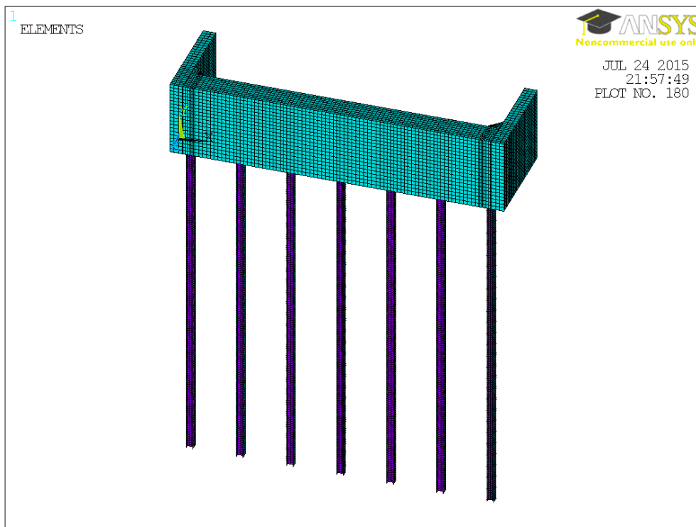
Figure 9-7 Finite element model of an integral abutment bridge with U-shaped cantilever wingwalls
