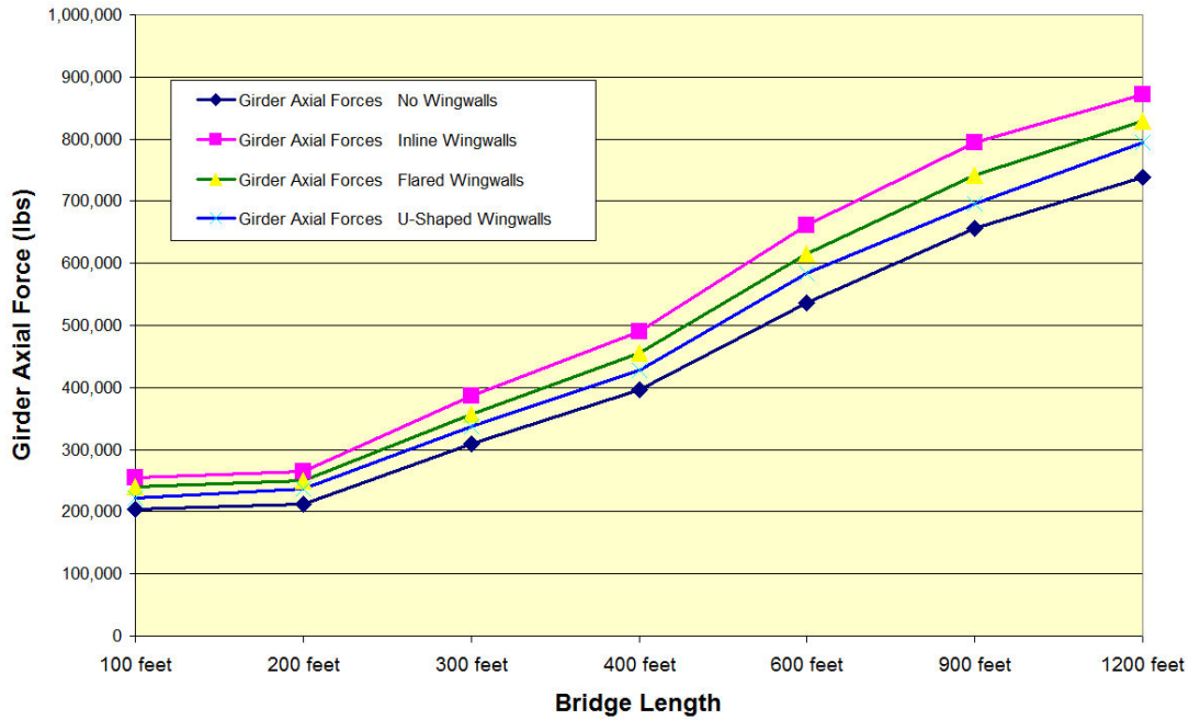
Figure 10-21 Girder axial forces during temperature expansion using dense sand backfill soil and predrilled holes at the top nine feet of piles
