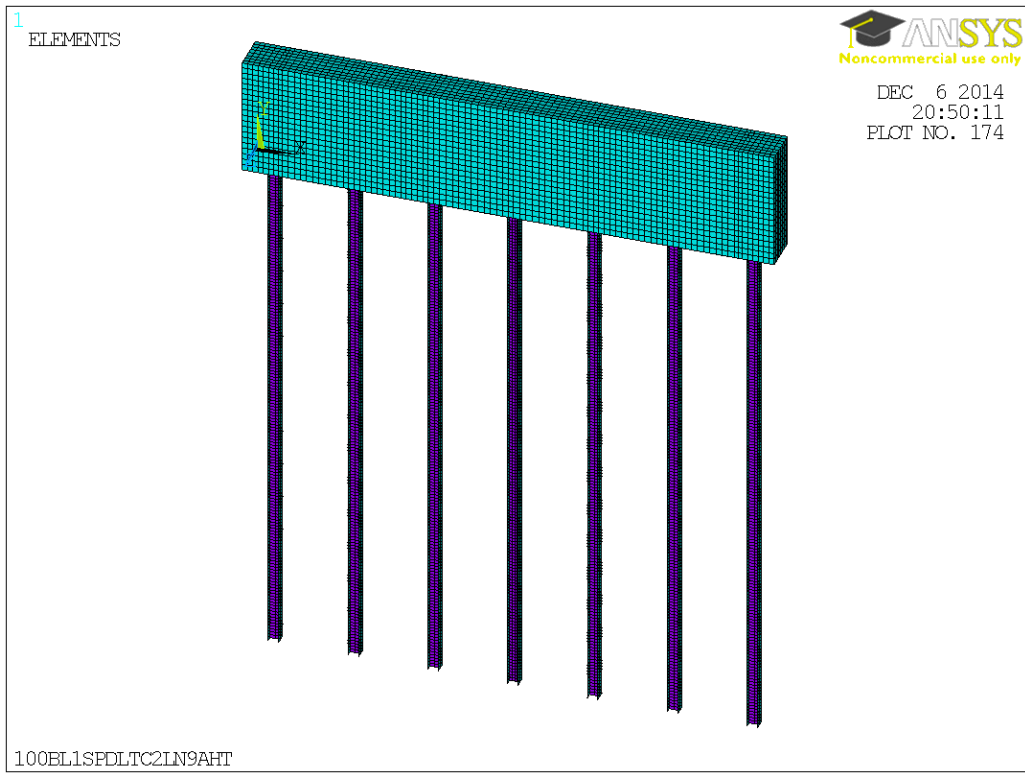
Figure 9-4 Finite element model of an integral abutment bridge with no cantilever wingwalls
