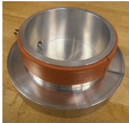
Figure 2.16 Vapor containment end caps and closed cell foam
