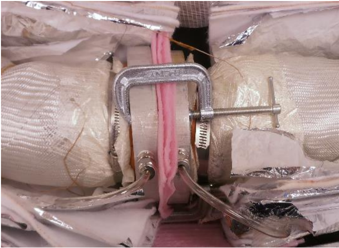
Figure 2.17 End caps with ends of plastic and fiberglass secured
