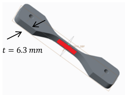
Figure 6.1. Specimen geometry (sizes are in mm)
