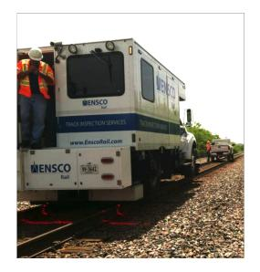
Figure 4.4: CTIV platform used to collect the images.
