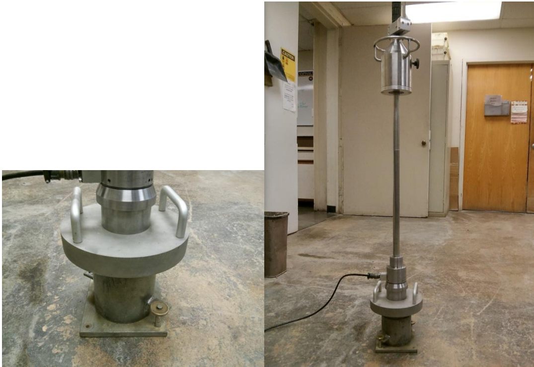
Figure 2.36. Configuration of Olson LWD test on top of the Proctor mold. (Tefa, 2015)
