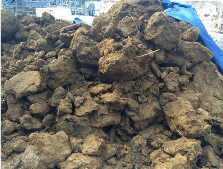
Figure 3.6. Stockpile of HPC soil
