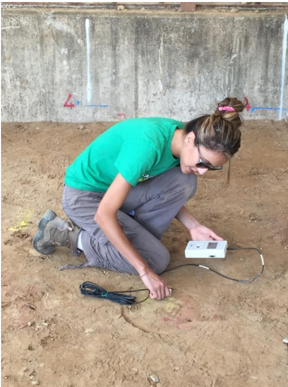
Figure 4.5. Decagon GS1 VWC sensor inserted from the top on the ALF soil; VWC reading with ProCheck
