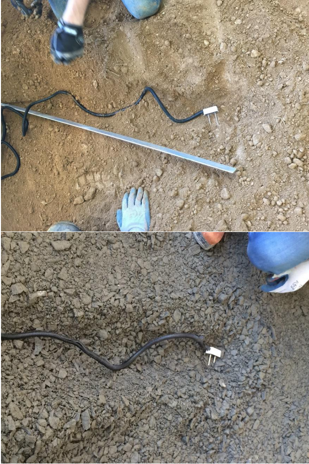
Figure 4.9. Embedding the GS1 VWC sensor in ALF and VA21a soil
