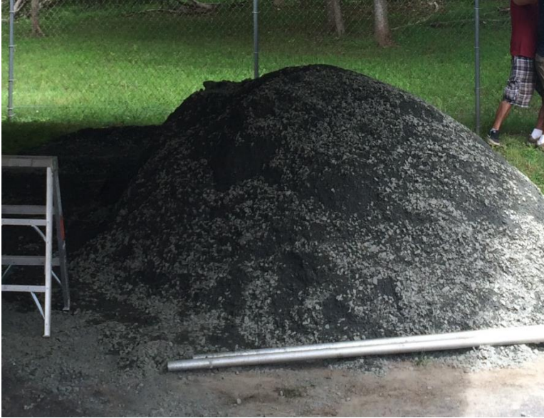
Figure 3.8. Stockpile of VA21a stone
