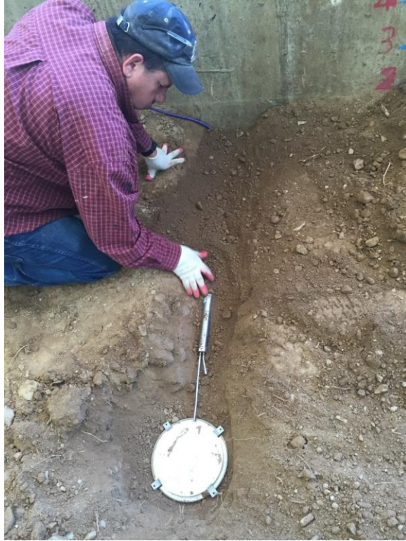
Figure 4.14. Embedding the pressure cell in the ALF soil Pit 1
