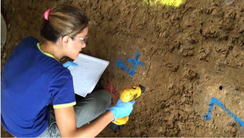
Figure 4.6. Use of drill to prefabricate holes for the Decagon GS1 VWC sensor insertion into HPC soil
