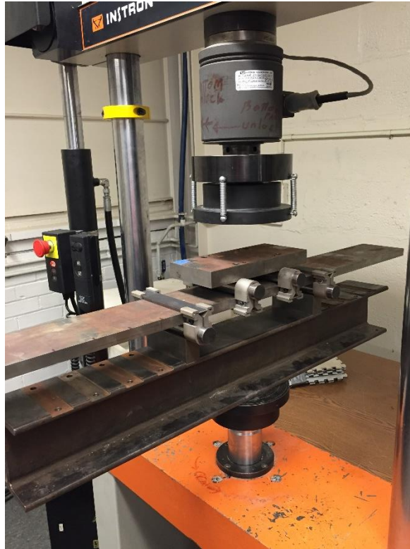
Figure 2.13. measurement of BVT static stiffness ( k_s ) with the Instron machine
