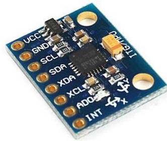
Figure 3.4.1: MPU 6050 Gyroscope. Image retrieved from http://www.digibay.in/
