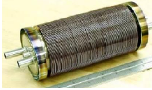
(b) Coiled tube-in-shell counter-flow recuperator in a miniature Brayton cryocooler (Zagarola and McCornick, 2006)
