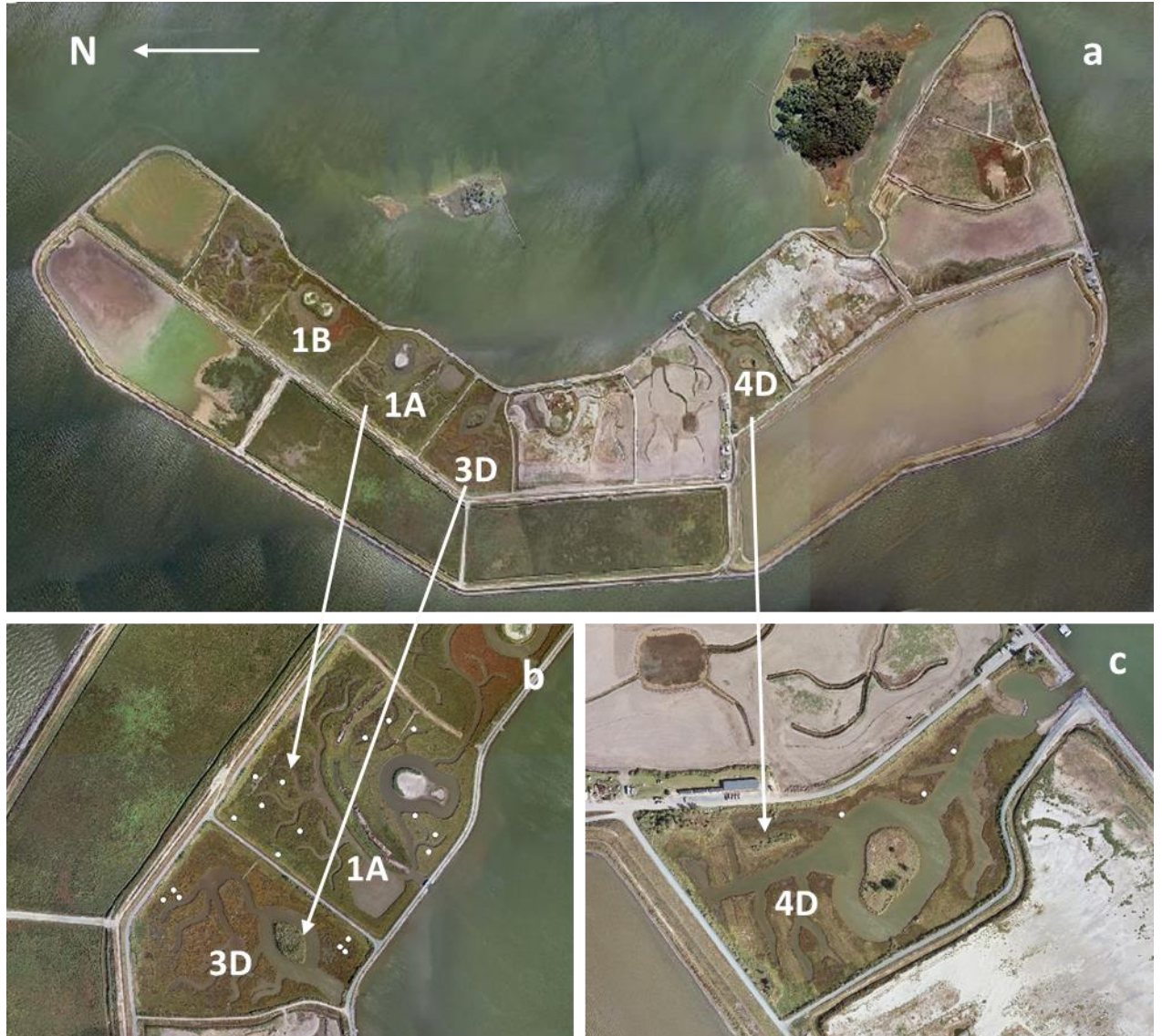
Figure 2-3. Aerial photograph of Poplar Island (September 2014), showing containment cells (Cells 1B, 1A, 3D, 4D) being developed as tidal marsh habitat on the east side of the island (a). Locations of rSETs used in this study are indicated by white dots in images (b) and (c).
