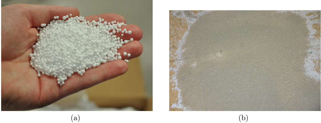
Figure 7.1: Images of granular materials in the laboratory. (a) bean-bag chair particles (expanded polystyrene). (b) spill of 750–1000 \mu\text{m} diameter glass spheres on the floor and spread out a bit with a broom before being cleaned up (slipping hazard).
