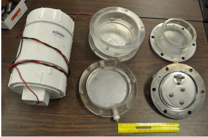
Figure 8.3: The three cells that have been used 2011–2015. The first cell (left), hand-shaken and filled with sand, developed by Paul Lathrop and Daniel Lathrop. The second cell (middle), shaken using the linear motor, was developed and used by Zack Lasner and Julia Salevan (Salevan 2012). The third and current cell (right), able to hold a partial vacuum, was developed and originally used by Tyler Holland-Ashford and Allison Bradford. The yellow ruler in the image is 15 cm long.
