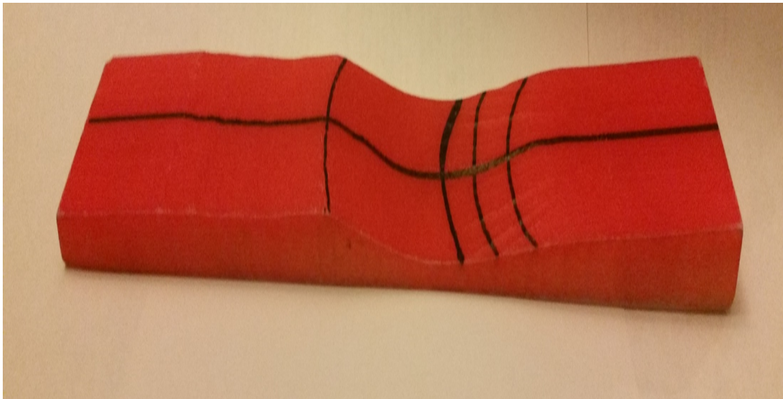
Figure 3.11: Prototype bedform used in single-phase measurements.
