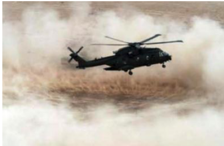
Figure 2.1: Formation of a dust cloud in the landing zone, Johnson et al. (2010)
