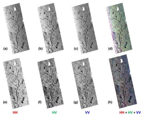
Figure 3-9. Polarized AIRSAR image acquired on 1994/10/07 in three polarizations and composite (R: HH, G: HV, B: VV). The above images (a)-(d) show the image requested from JPL archive, and the below images (e)-(h) are after correction for incident angle.
