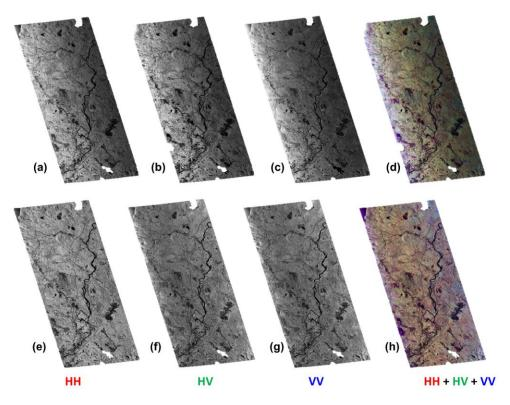
Figure 3-10. Polarized UAVSAR image acquired on 2009/08/05 in three polarizations and composite (R: HH, G: HV, B: VV). The above images (a)-(d) show the calibrated image distributed by JPL, and the below images (e)-(h) are after correction for incident angle.
