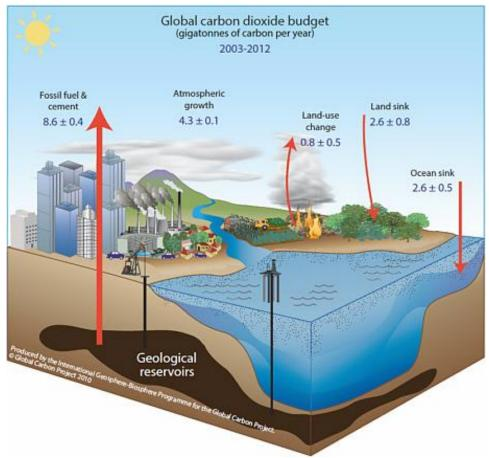
Figure 1-1. Conceptual diagram of global carbon dioxide budget. Global Carbon Project 2014 (Le Quere et al., 2014).
