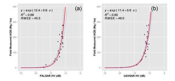
Figure 4-10. Errors from regression models: (a) PALSAR 2009 HV, (b) UAVSAR 2009 HV. Y axis is the field measured AGB density (Mg·ha<sup>-1</sup>) at 1.0 ha plot-level. X axis is SAR backscatter at HV polarization in decibel (dB). Red solid line is the prediction curve, and blue dashed lines are the 95% confidence intervals of predictions.
