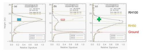
Figure 2-4. Typical co-incidence waveforms (center within 2m) from LVIS 2003 and 2009 data. (a) RHs relatively unchanged; (b) RHs have significant negative changes; (c) RHs with positive change. Black solid waveform is from 2009, gold dash waveform is from 2003. Red solid line is the detected ground in LGE, dashed straight lines are the RH100, dashed with dot lines are the RH50.
