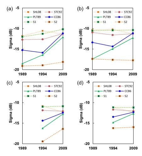
Figure 3-13. Original and normalized multi-sources backscatter (1989–2009) from airborne- and spaceborne- SAR systems at represented stands: (a) and (c) are from original data, and (c) and (d) are from normalized data. Airborne data include AIRSAR 89/09/02, 94/10/07, and UAVSAR 09/08/05. Spaceborne data include SIR-C/XSAR 94/10/07 and PALSAR 09/08/30.
