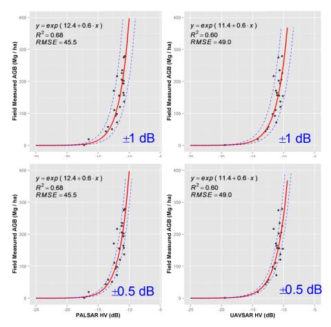
Figure 4-9. Simulated errors from SAR datasets: (a) PALSAR 2009 HV with  $\pm 1$  dB error, (b) UAVSAR 2009 HV with  $\pm 1$  dB error, (c) PALSAR 2009 HV with  $\pm 0.5$  dB error, and (d) UAVSAR 2009 HV with  $\pm 0.5$  dB error. Red solid line is the fitted regression model, and blue dashed lines show the SAR calibration error interval.
