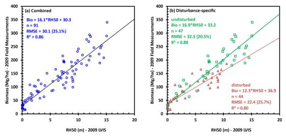
Figure 2-7. Relationship between field biomass and LVIS relative height metric RH50 at footprint-level: (a) Combined model; (b) Disturbance-specific models. Different colors indicate different models: rectangle dots (green) represent the undisturbed group, and triangle dots (red) represent the disturbed group.
