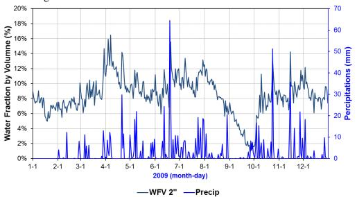
Figure 3-3. Water fraction by Volume (WFV, %) and precipitation (mm) as a function of date. WFV measured at depths of 2 inches (~=5 cm).
