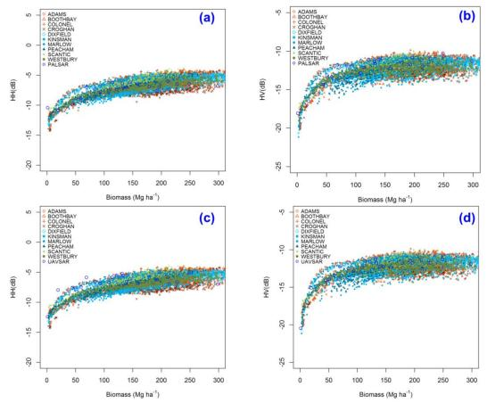
Figure 3-5. SAR backscatter as a function of forest aboveground biomass from model simulation and remote sensing observation. Simulation from ZELIG plotted with (a) PALSAR HH, (b) PALSAR HV, (c) UAVSAR HH, and (d) UAVSAR HV. ADAMS to WESTBURY are different type of soil based on drainage and taxonomic classification (Levine et al., 1994).
