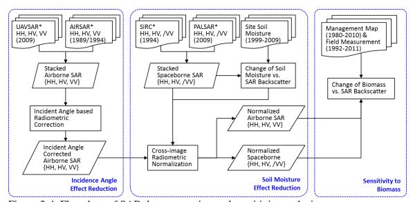
Figure 3-4. Flowchart of SAR data processing and sensitivity analysis.
