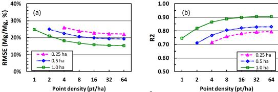
Figure 2-14. Sensitivity of RMSE% (a) and R<sup>2</sup> (b) to the density of footprints within the plot (pt ha<sup>-1</sup>) at 0.25 ha, 0.5 ha and 1.0 ha plot-levels; RMSE (%) and R<sup>2</sup> values were from the combined RH50 footprint-level biomass prediction model.
