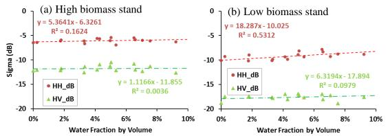
Figure 3-11. Mean backscatter (Sigma) plotted as a function of water fraction by volume (WFV, %): (a) High biomass stand, (b) Low biomass stand.
