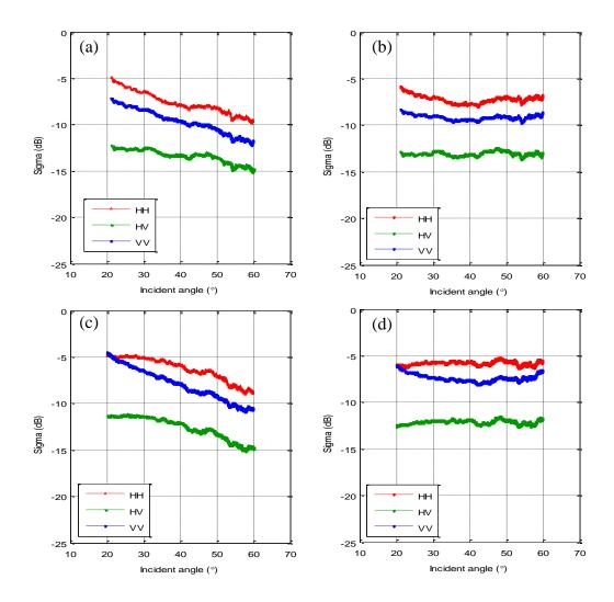
Figure 3-8. Mean backscatter in three polarizations (R:HH, G:HV, B: VV) as a function of incidence angle. AISSAR data acquired on 10/07/1994before (a) and after incidence angle normalization (b), UAVSAR data acquired on 08/05/2009 before (c) and after incidence angle normalization (d).
