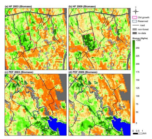
Figure 2-10. Biomass map for HF site (a) and (b), and PEF site (c) and (d) in 2003 and 2009 at 1.0 ha level by the combined RH50 models. A color of orange to dark green indicates an increase of biomass. At HF site, pink polygon is near matured oldgrowth forest; and dark blue polygon is the outline of reserve area.
