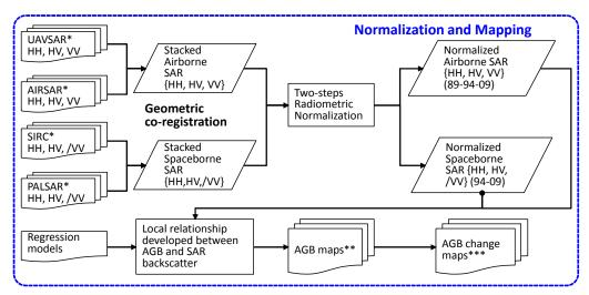
Figure 4-2. Flowchart of SAR data preparation, normalization and mapping.
