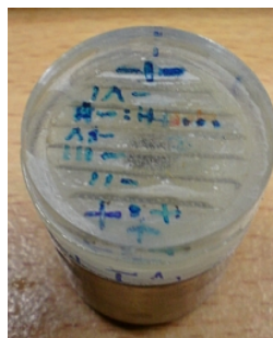
Fig 58: Isometric view of work cylinder with six acrylic strips fixed on top of it..
