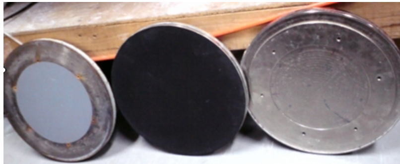
Fig 65: Real object of the stainless steel lapping/polishing plates we designed.
