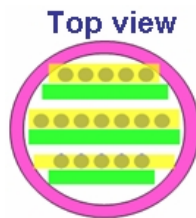
Fig 30: Top view of the layout of capillary arrays fixed on top of work cylinder.
