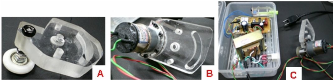
Fig 85: (A) enlarged view of the short jig arm (B) enlarged view of the motor jig assembly (C) Motor speed controller and its assembly
