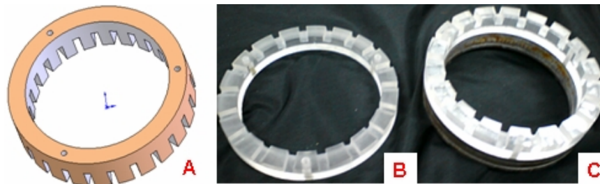
Fig 79: (A) 3D plot and (B) photo of work ring of small diameter
