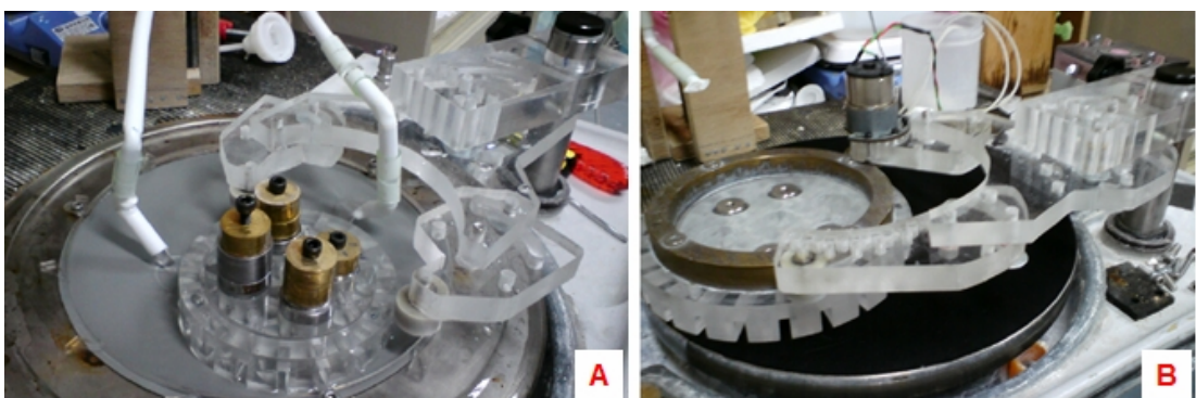
Fig 86: (A) flexible acrylic swing jig holder operates for small workpiece fixture. (B) flexible acrylic swing jig holder operates for large workpiece fixture.
