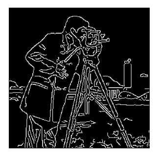
Figure 4.1: Output of the Canny algorithm on the cameraman image. Detected edges are in white.
