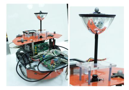
(a) Dr. Robot Platform (b) Parabolic Mirror Figure 6.1: Test Platform
