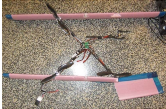
FIGURE 5.10: Vehicle damaged during flight tests
