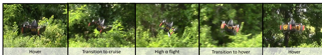
FIGURE 7.13: AirEZ-Micro outdoor flight testing ( https://www.youtube.com/watch?v=p4jwYw_LV6M )
