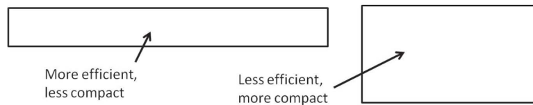
FIGURE 3.6: Wing aspect ratio trade-off: efficiency and compactness
