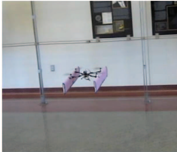
FIGURE 5.6: Quad-rotor biplane in hover
