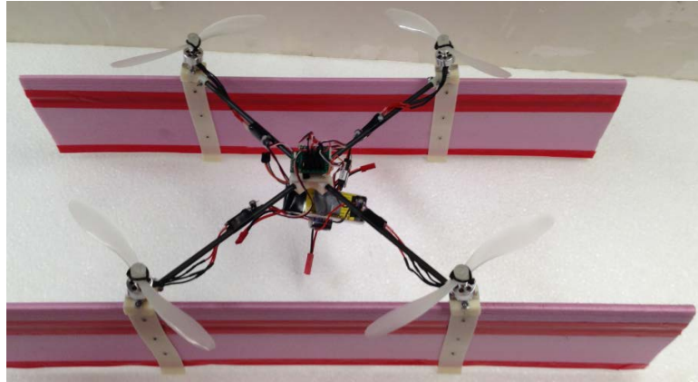
FIGURE 6.3: Vehicle with 3D printed motor mounts
