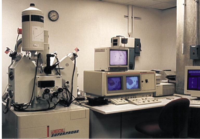
Figure 1-7 Image of a JOEL 8900 WDS/EDS microprobe used in the composition measurement of the alloy thin film samples for this study. Image from [44].
