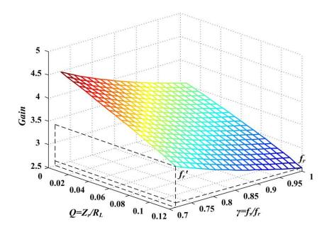
Figure 2.7. Voltage gain characteristics of the resonant converter.
