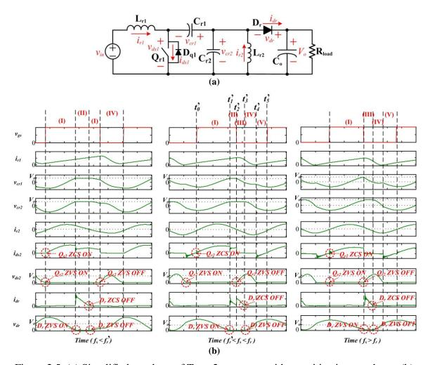
Figure 2.5. (a) Simplified topology of Type 2 converter with a positive input voltage; (b) The voltage and current waveforms of Type 2 converter with a positive input voltage and different switching frequencies.
