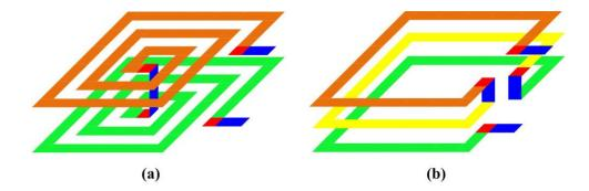
Figure 1.22. 2D stacked planar layouts: (a) stacked spiral coils with same direction, and (b) multilayer coils with different directions [131].
