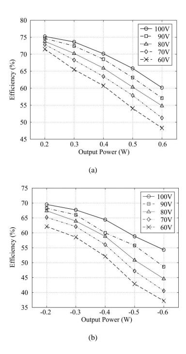
Figure 4.14. Conversion efficiency versus output power of the resonant converter at different output drive voltages: (a) boost mode; (b) buck mode.
