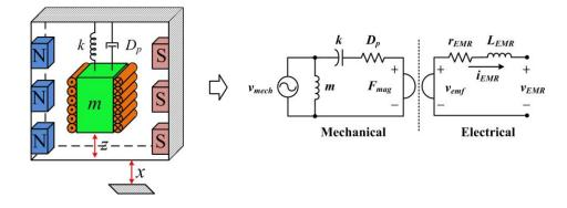
Figure 3.1. Equivalent circuit of one EMR generator ( $v_{mech}$ : mechanical velocity; *m*: proof mass; *k*: spring stiffness;  $D_p$ : mechanical damping;  $F_{mag}$ : magnetic force;  $v_{emf}$ : EMF;  $r_{EMR}$ : coil resistance;  $L_{EMR}$ : self-inductance;  $i_{EMR}$ : generator terminal current;  $v_{EMR}$ : generator terminal voltage).
