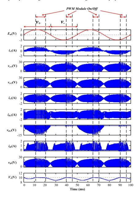
Figure 2.12. Simulation waveforms of Type 1 converter with 2-Vrms alternating input voltage, using module on/off control.
