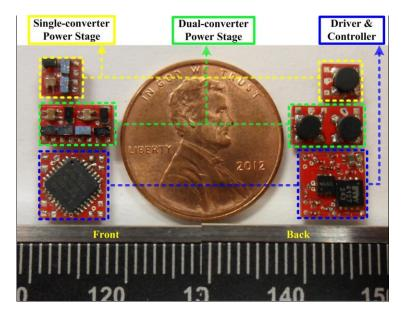
Figure 4.12. Front ( $L_{in}$ ,  $C_{r1}$ ,  $C_{r2}$ ,  $Q_{r1}$  and  $Q_{r2}$ ) and back ( $L_p$  and  $L_s$ ) views of 100-mg, 1.5-MHz experimental prototype of the paralleled resonant dc-dc converters, as well as its driver and controller.
