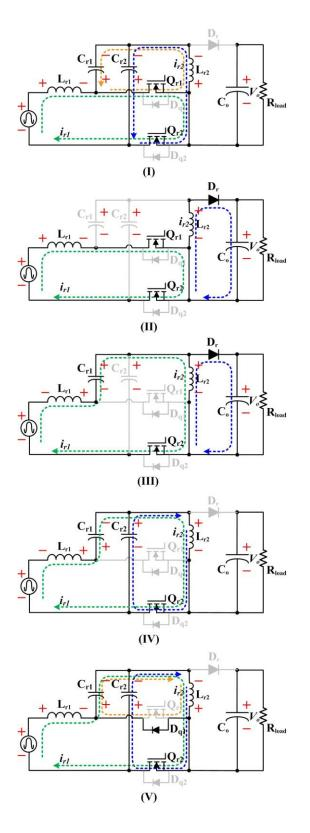
Figure 2.3. Switching sub-intervals for Type 2 converter with a positive voltage input source, during one switching cycle.
