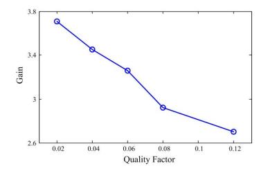
Figure 2.16. Voltage gain of Type 1 converter at  $+3V_{dc}$  input under different load conditions.
