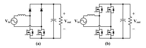
Figure 1.5. Single-stage H-bridge ac-dc converters: (a) two-switch boost converter [63] and (b) four-switch boost converter [64].
