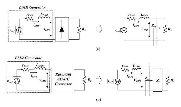
Figure 3.3. Impedance network of an EMR generator interfaced with (a) a diode bridge; and (b) a single-input resonant ac-dc converter ( $Z_r$ : characteristic impedance;  $R_{load}$ : load resistance;  $Z_{in}$ : equivalent input impedance).
