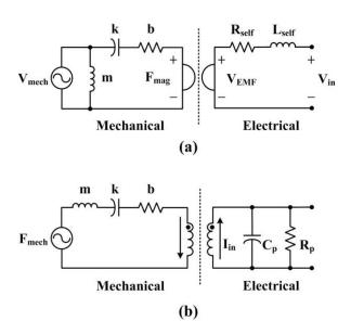
Figure 1.1. Equivalent circuits of generators: (a) EMA generators (v<sub>mech</sub>: mechanical velocity, m: proof mass, k: spring stiffness, b: damping, F<sub>mag</sub>: magnetic force, V<sub>EMF</sub>: EM force, R<sub>self</sub>: coil resistance, L<sub>self</sub>: self-inductance); and (b) PZ generators (F<sub>mech</sub>: stress, m: mass, k: stiffness, b: damping, I<sub>in</sub>: induced current, C<sub>p</sub>: shunt capacitance, R<sub>p</sub>: shunt resistance) [18].
