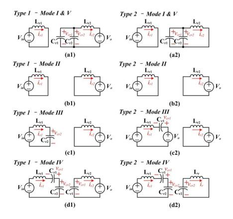
Figure 2.6. The equivalent circuit models of Type 1 converter: (a1) corresponding to Stages I and V; (b1) Stage II; (c1) Stage III; (d1) Stage IV. The equivalent circuit models of Type 2 converter: (a2) corresponding to Stages I and V; (b2) Stage II; (c2) Stage III; (d2) Stage IV.
