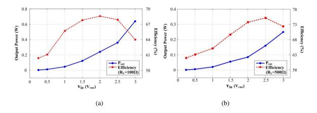
Figure 2.20. Open-loop output power and efficiency over input voltage of Type 1 converter at (a)  $R_{load}$ =100  $\Omega$ ; and (b)  $R_{load}$ =500  $\Omega$ .
