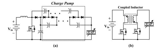
Figure 1.16. Single-stage converters: (a) a boost converter cascaded with a charge pump circuit [108], and (b) a bidirectional flyback converter [110].
