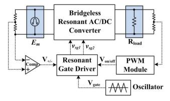
Figure 2.10. Block diagram of module on/off control and polarity identification for resonant switching and gating.
