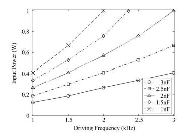
Figure 4.15. Input power demands of the converter at different driving frequencies and load capacitances.
