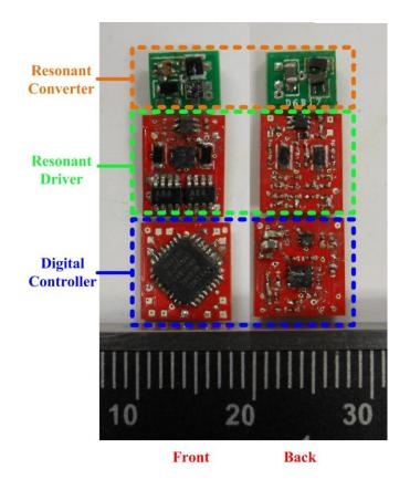
Figure 2.13. Front ( $L_{r1}$ ,  $C_{r1}$ ,  $C_{r2}$ ,  $Q_{r1}$  and  $Q_{r2}$ ) and back ( $L_{r2}$ ,  $D_r$  and  $C_o$ ) views of 100-mg, 2-MHz experimental prototype of the proposed Type 1 resonant ac-dc converter, as well as its resonant driver and digital controller.
