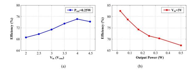
Figure 2.21. Closed-loop efficiency over (a) input voltage (at  $P_{out}=0.25$  W); and (b) output power (at  $V_{in}=3$  V<sub>rms</sub>).
