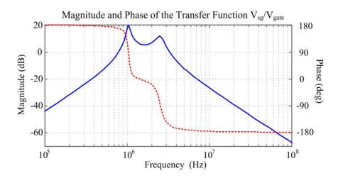
Figure 2.9. Frequency response of the transfer function of the resonant tank.
