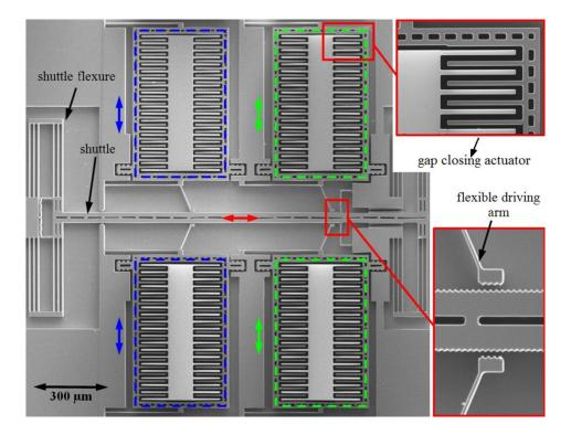
Figure 4.17. SEM image of the electrostatic actuators for inchworm motor [8].
