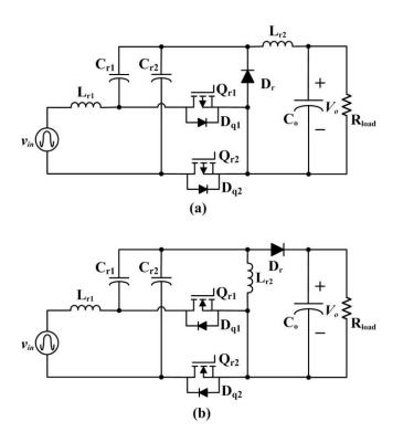
Figure 2.1. Proposed bridgeless resonant ac-dc step-up converters: (a) Type 1; (b) Type 2.
