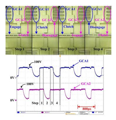
Figure 4.18. Dynamic driving performance of two sets of GCAs during one alternative driving cycle.
