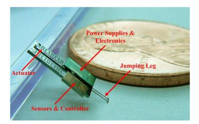
Figure 1.2. Mock-up of a jumping microrobot [112].
