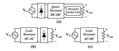
Figure 1.15. Soft-switching converters: (a) diode bridge cascaded with quasi-resonant dcdc converter; (b) load-resonant ac-ac converter cascaded with diode bridge; (c) bridgeless resonant ac-dc converter.
