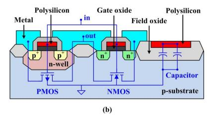
Figure 1.19. CMOS integrated circuit: (a) CMOS inverter, (b) cross-sectional schematic of two transistors and capacitors die chip, in an n-well CMOS process [123].
