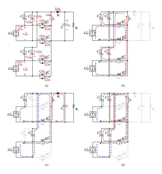
Figure 3.5. (a) Simplified topology of dual-input resonant converter with a positive input and a negative input; (b)~(d) switching sub-intervals during a switching cycle.
