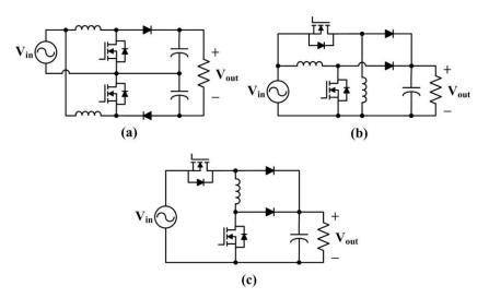
Figure 1.6. Single-stage bridgeless ac-dc converters: (a) bridgeless boost converter [65],(b) bridgeless buck-boost converter [66], and (c) bridgeless switched-inductor boost converter [67].
