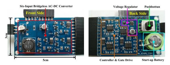
Figure 3.11. Six-input standalone prototype of the proposed resonant ac-dc converter for a six-EMR-generator system.
