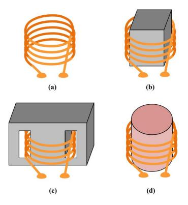
Figure 1.23. 3D solenoid layouts: (a) micro-coil with air [133], (b) micro-coil with openloop magnetic core, (c) micro-coil with closed-loop magnetic core, and (d) micro-coil with non-magnetic core [134].
