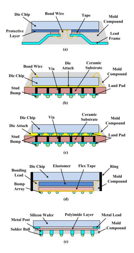
Figure 1.20. Cross-sectional view of CSP: (a) lead frame based CSP, (b) rigid substrate based CSP with wire bonding, (c) rigid substrate based CSP with flip-chip, (d) flexible substrate based CSP, and (e) wafer-level CSP [125].
