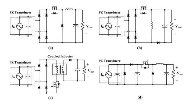
Figure 1.9. Resistive impedance matching converters: (a) diode full bridge followed by buck converter [73], (b) diode full bridge followed by buck-boost converter [74], (c) diode full bridge followed by flyback converter [75], and (d) voltage multiplier followed by buck converter [76].
