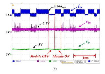
Figure 2.18. Closed-loop experimental waveforms of Type 1 converter operating with (a) voltage regulation for  $V_o=5$  V,  $R_{load}=100 \Omega$ ; (b) module on/off control at 20-kHz modulation frequency.
