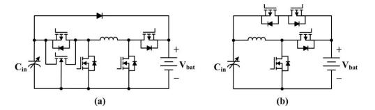
Figure 1.14. Battery constrained converters: (a) switched inductor buck-boost converter [86] and (b) switched inductor boost converter [87].
