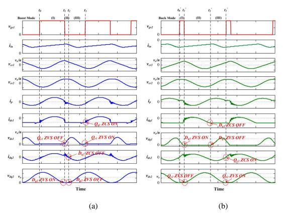
Figure 4.5. The voltage and current waveforms of the proposed converter during (a) boost mode (actuator drive), and (b) buck mode (energy recovery).
