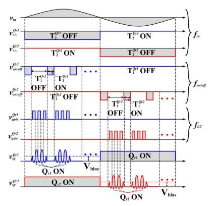
Figure 2.11. Resonant gating signal corresponding to on/off control signal and polarity identification signal, in the case of Type 1 converter.
