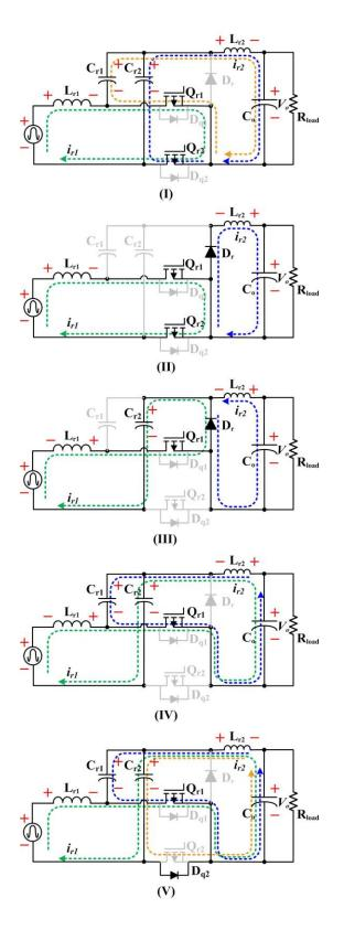
Figure 2.2. Switching sub-intervals of Type 1 converter with a positive voltage input source, during one switching cycle.
