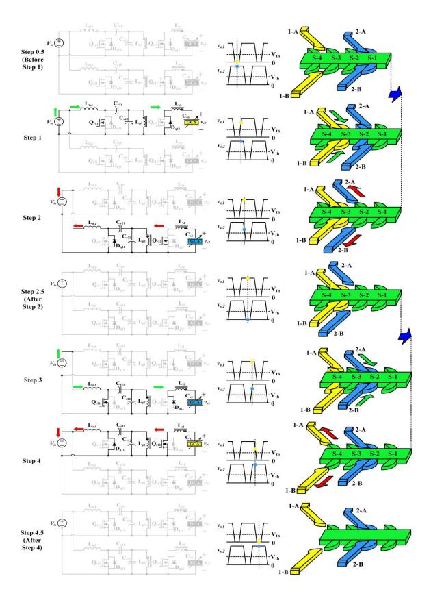
Figure 4.9. Alternative strategy for driving electrostatic multi-GCA inchworm motor.
