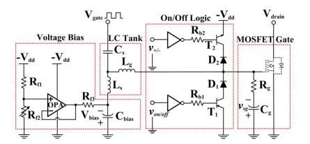
Figure 2.8. Resonant gate drive circuit for Type 1 converter.
