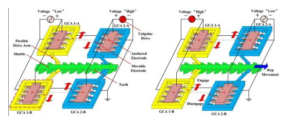
Figure 4.2. Electrostatic inchworm motor driven by two anti-phase drive signals.
