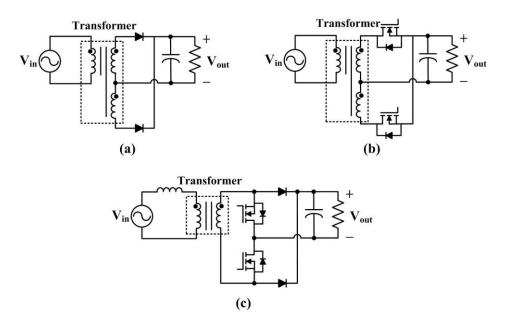
Figure 1.8. Single-stage transformer-based rectifier: (a) center-tapped transformer fullwave passive rectifier, (b) center-tapped transformer full-wave phase controlled rectifier [71], and (c) transformer-based active boost rectifier [72].
