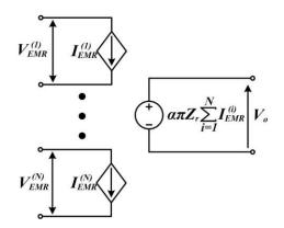
Figure 3.7. Switching average model of an *N*-channel system.
