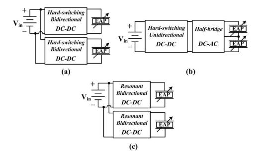
Figure 1.18. Topologies for driving multiple EAP actuators: (a) paralleling bidirectional dc-dc switching converters, (b) a unidirectional dc-dc converter cascaded with half-bridge inverters, (c) paralleling bidirectional resonant converters.
