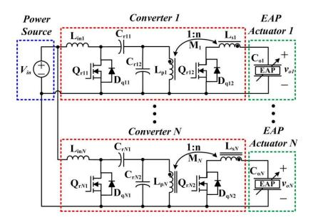
Figure 4.8. Paralleled topology for driving multiple EAP actuators.
