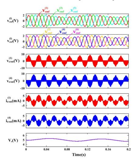
Figure 3.10. Simulation waveforms of a six-input converter connected to a resistive load.
