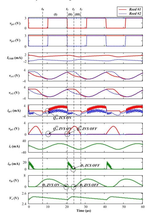
Figure 3.6. Simulation waveforms of dual-channel system during a switching cycle.
