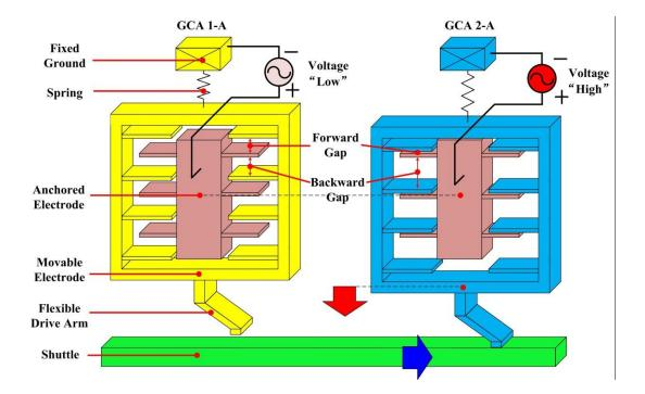
Figure 4.1. Mechanism of in-plane electrostatic gap-closing actuators (GCA) at one side of the shuttle.
