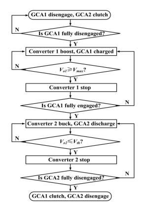
Figure 4.10. Logical flow chart of the alternative driving strategy during a half driving cycle.
