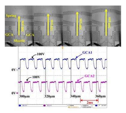
Figure 4.19. Dynamic motion of the shuttle of the inchworm motor during alternative driving process.
