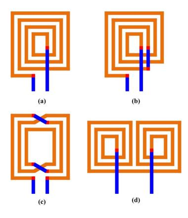
Figure 1.21. 2D spiral planar layouts: (a) conventional spiral, (b) conventional spiral with equal loop area, (c) interwound spiral, and (d) twin spiral [130].
