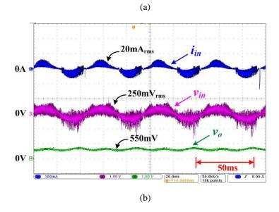
Figure 2.17. Open-loop experimental waveforms of Type 1 converter operating with (a)  $V_{in}$ =3 V<sub>rms</sub> (20 Hz, ac),  $V_o$ =7.6 V (dc),  $R_{load}$ =100  $\Omega$ ; (b)  $V_{in}$ =0.25 V<sub>rms</sub> (20 Hz, ac),  $V_o$ =0.55 V (dc),  $R_{load}$ =100  $\Omega$ , during 2-MHz switching:  $i_{in}$ ,  $v_{in}$  and  $V_o$ .
