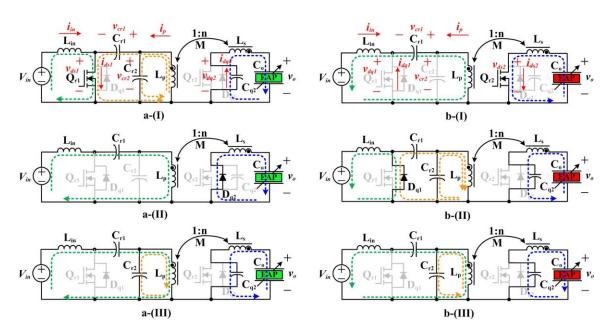
Figure 4.4. a-(I)~a-(III) Equivalent circuits corresponding to the switching sub-intervals during boost operation (driving actuators); b-(I)~b-(III) equivalent circuits corresponding
