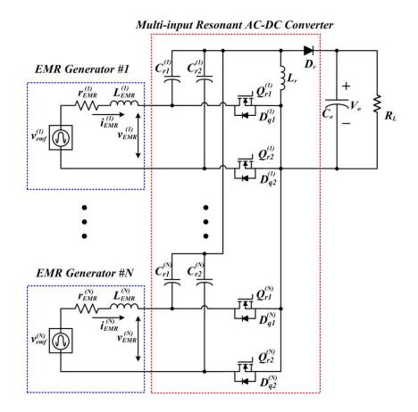
Figure 3.4. Illustrative scheme of the proposed multi-input converter  $(v^{(i)}_{emf})$  EMF of #i channel;  $r^{(i)}_{EMR}$ : coil resistance;  $L^{(i)}_{EMR}$ : self-inductance;  $i^{(i)}_{EMR}$ : channel terminal current;  $v^{(i)}_{EMR}$ : channel terminal voltage;  $C^{(i)}_{r1} = C^{(i)}_{r2}$ : resonant capacitors;  $L_r$ : resonant inductor;  $Q^{(i)}_{r1}$ ,  $Q^{(i)}_{r2}$ : MOSFETs;  $D_r$ : output diode;  $C_o$ : output capacitor).
