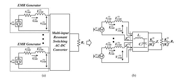
Figure 3.8. (a) An *N*-channel EMR generator system connected with an *N*-input resonant ac-dc converter; and (b) impedance network of an *N*-channel system.
