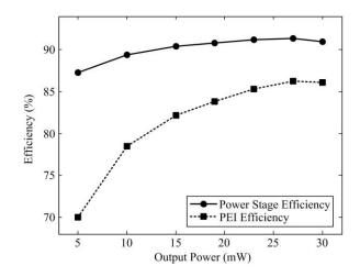
Fig. 3.15. Power conversion efficiency of the power stage and the entire PEI (including controller losses) at different output power.
