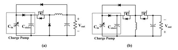
Figure 1.13. Voltage constrained converters: (a) charge pump buck flyback converter [84] and (b) charge pump buck-boost flyback converter [85].
