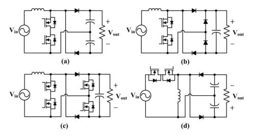
Figure 1.7. Single-stage bridgeless bidirectional switch ac-dc converters: (a) split outputcapacitor boost converter, (b) auxiliary diode boost converter, (c) auxiliary switch boost converter, and (d) split output-capacitor buck-boost converter [68]-[70].
