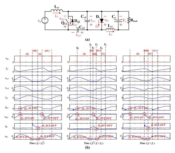
Figure 2.4. (a) Simplified topology of Type 1 converter with a positive input voltage; (b) The voltage and current waveforms of Type 1 converter with a positive input voltage and different switching frequencies.
