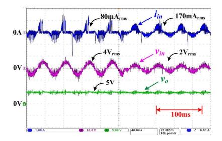
Figure 2.19. Closed-loop dynamic response of Type 1 converter operating with voltage regulation for  $V_o=5$  V,  $R_{load}=100 \Omega$ .
