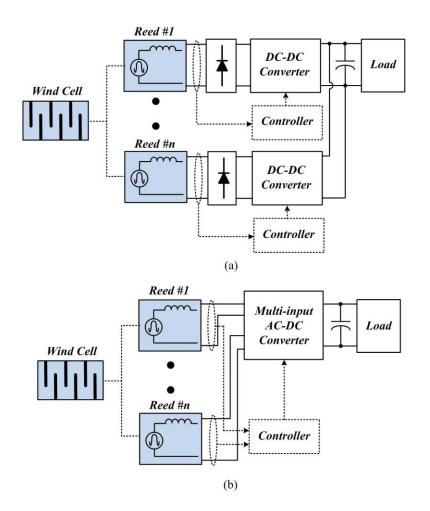
Figure 3.2. Multiple EMR generators and PEI system: (a) conventional PEI; and (b) proposed multi-input PEI.
