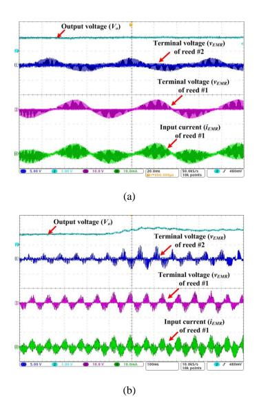
Figure 3.16. Experimental waveforms of EMR generators: X-axis: (a) 20 ms/div; (b) 100 ms/div; Y-axis: (a) constant wind speed; (b) wind speed step change; Ch1 = terminal voltage ( $v_{EMR}$ ) of channel #2, 5 V/div; Ch2 = output voltage ( $V_o$ ), 1 V/div; Ch3 = terminal voltage ( $v_{EMR}$ ) of channel #1, 10 V/div; Ch4 = input current ( $i_{EMR}$ ) of channel #1, 10 mA/div.
