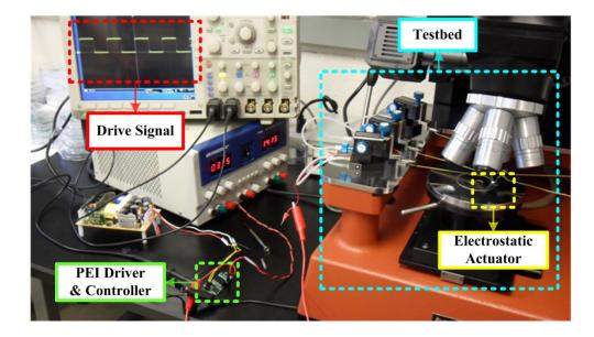
Figure 4.16. Electrostatic actuator driving test by utilizing the adopted PEI driver (500 mW, 63 mg, 31.5 mm<sup>2</sup>) and its controller [112].
