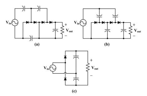
Figure 1.4. Voltage multiplying rectifiers: (a) Villard voltage multiplier [60], (b) Dickson voltage multiplier [61], and (c) bridge voltage doubler rectifier [62].
