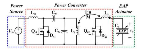
Figure 4.3. Proposed bidirectional resonant dc-dc converters for driving EAP actuators.
