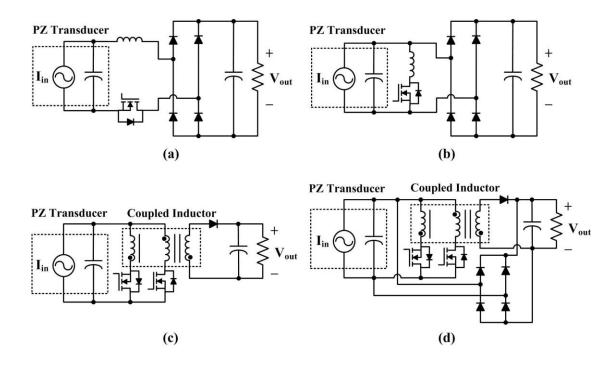
Figure 1.10. SSHI converters: (a) series-SSHI converter [77], (b) parallel-SSHI converter [78], (c) SSHI-MR converter [79], and (d) hybrid-SSHI converter [80].
