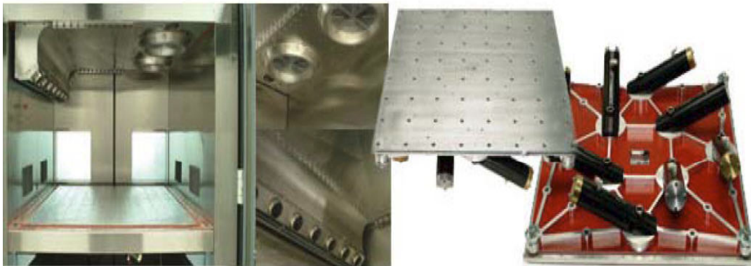
Figure 2-15. Typical RS Shaker Architecture
