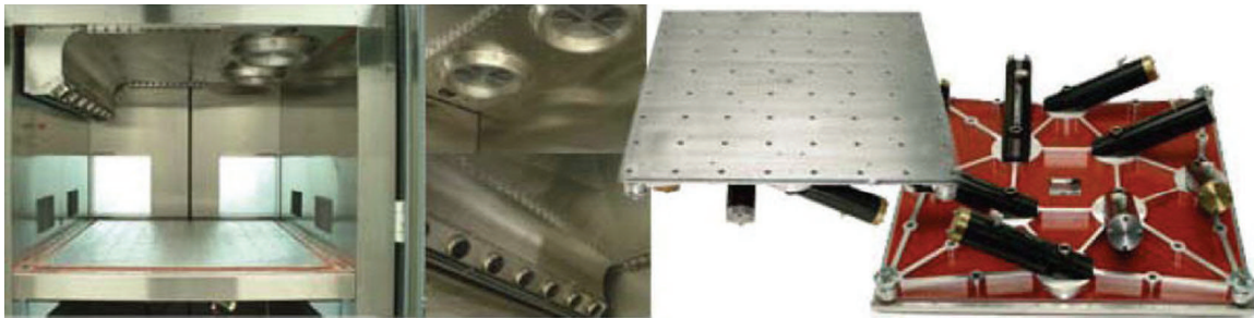
Figure 3-5. High accelerated life testing (HALT) chamber [15]
