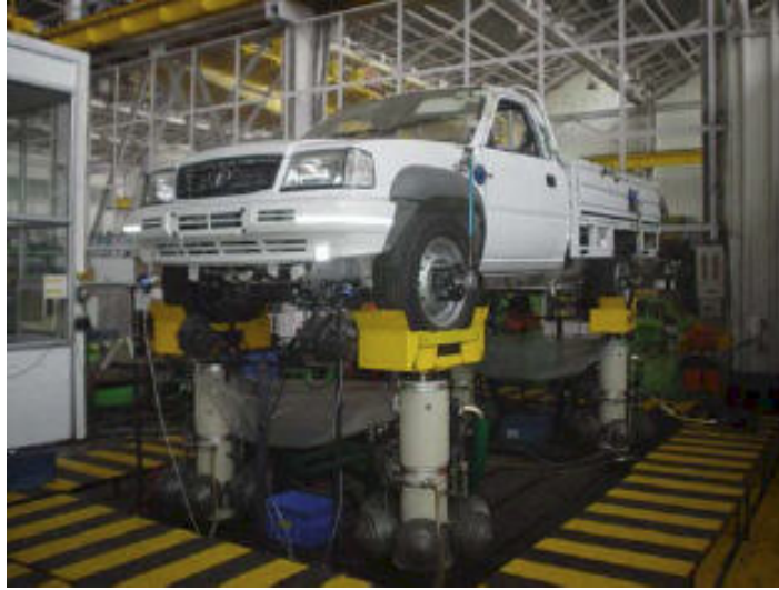
Figure 3-2. Four-post hydraulic simulator, from Awate et al. [17]
