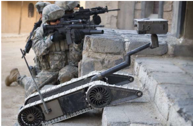
Figure 2-1. Small Unmanned Ground Vehicle (SUGV)
