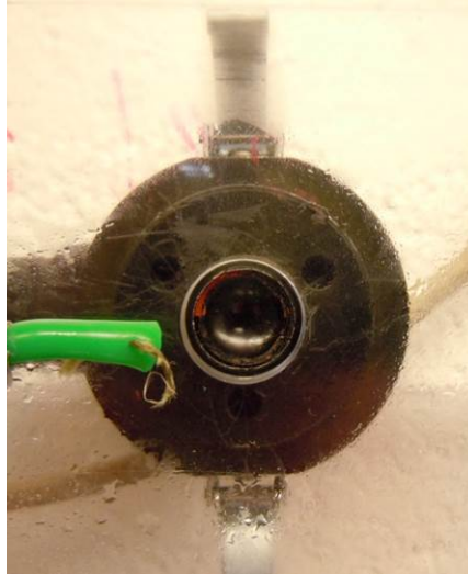
Figure 15: Design used to prevent accumulation of liquid on opacity meter lens
