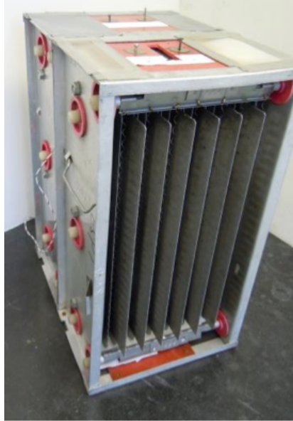
Figure 13: Geometry of wire-to-plate separator
