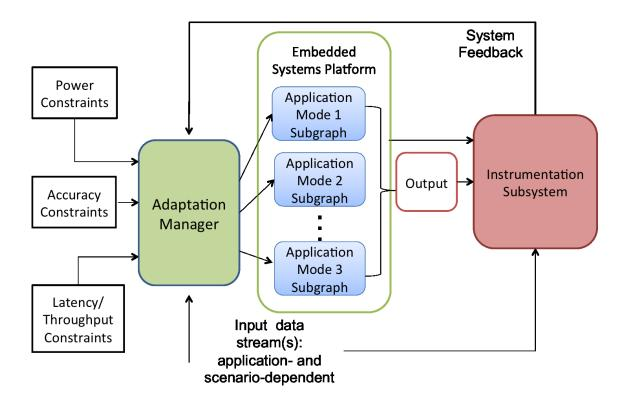
Figure 4.1: Data-driven, multi-mode embedded system design flow.
