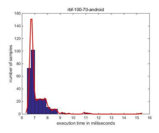
Figure 5.5: Task execution time for classifier subsystem 2.
