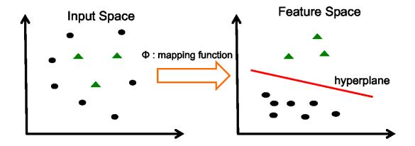
Figure 2.4: An illustration of an input space, feature space, and kernel function (mapping function) in SVMs.
