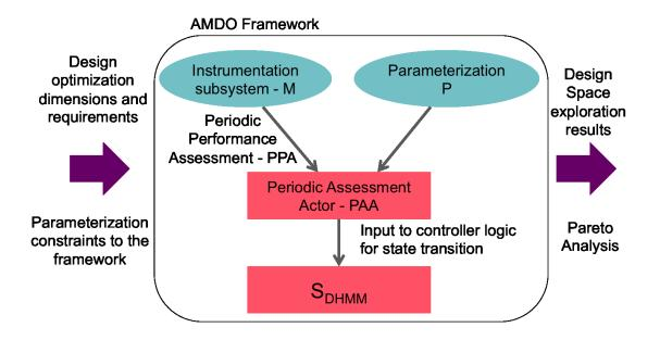
Figure 5.1: An overview of the adaptive multiobjective design optimization (AMDO) framework.
