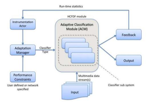
Figure 3.2: Overview of ASM system design in LiD4E.
