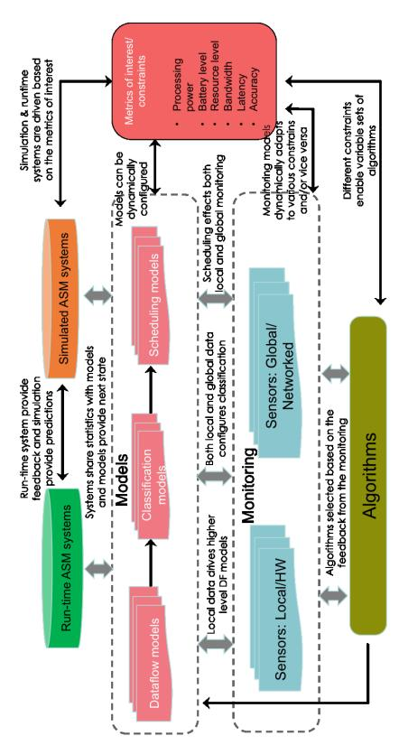
Figure 2.3: An illustration of the DDDAS paradigm applied to adaptive stream mining systems.
