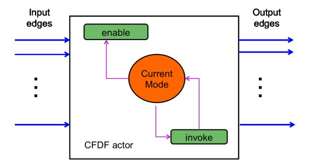
Figure 2.1: An illustration of a CFDF actor.
