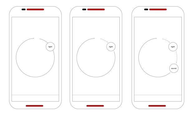
Figure 29: Drawing of the graphical state of the GPE after adding the light behavior, setting its activation condition, adding the sound behavior, and setting it's activation condition.
