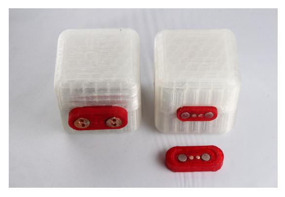
Figure 34: Photograph of the final prototype, showing the interchangeable port adapters, both attached (left) and detached (right) from modules.
