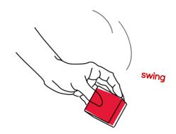
Figure 40: Drawing of the swing gesture. The swing gesture starts an interactive dialogue with Pixel in which it can assist in creating, remapping, and removing I/O channels through additional gesturing and feedback.
