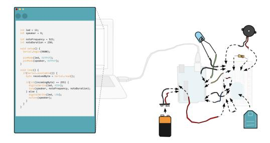
Figure 21: Drawing of connecting an additional "Output" device. This is done for each of the three additional devices. The complete program is shown in Figure 53 (Appendix A).
