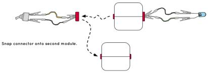
Figure 15: Drawing of the sequence of actions to adapt the light switch to be a remote light switch.
