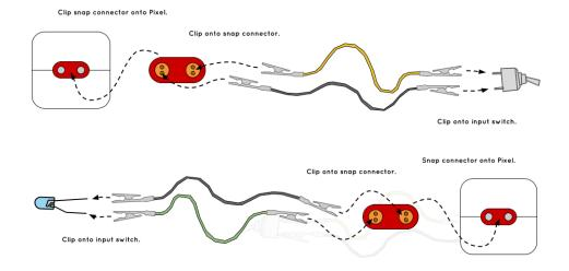
Figure 9: Drawing of connecting the input switch (top) and output LED (bottom) for the light switch. The complete system is shown in Figure 10.
