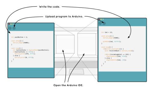
Figure 13: Drawing of the steps involved in programming the Arduino. The two separate Arduino sketches are shown to represent the two separate circuits in the remote light switch. The programming of both circuits needs to be updated. The complete sketches are shown in Figures 51 and 52 (Appendix A).
