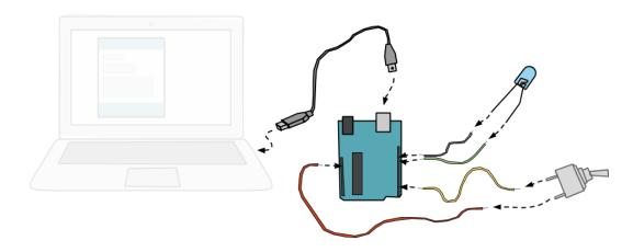
Figure 5: Drawing of connecting the components for the light switch.
