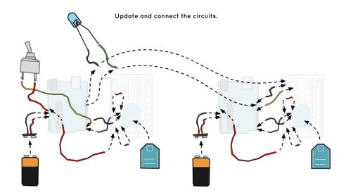
Figure 12: Drawing of the circuit connections and component placement on the breadboard for the remote light switch. Each dotted-line arrow represents a connection (and disconnection, for the LED) that must be made to update the circuits.
