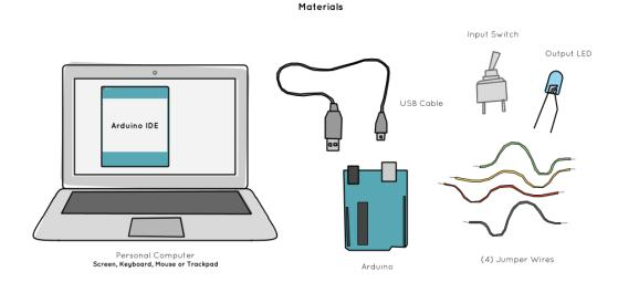
Figure 4: Illustration of the materials needed to make the light switch. Note that no current limiting resistor is used in this scenario, for simplicity.
