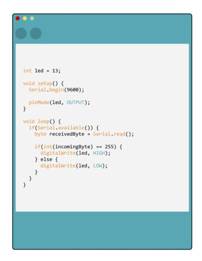
Figure 52: Drawing of the second Arduino program for the remote light switch in Example 2, Part 1. This corresponds to Figure 13.
