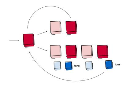
Figure 41: Illustration depicting the feedback behavior when the input switch is closed for the default behavior (top) and when a module's input maps to a different output module (bottom).
