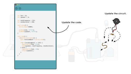
Figure 19: Drawing of connecting the speaker into the circuit and programming the circuit.
