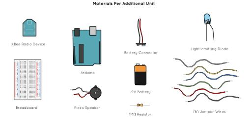
Figure 20: Illustration of the materials needed to create each additional "Output" device.
