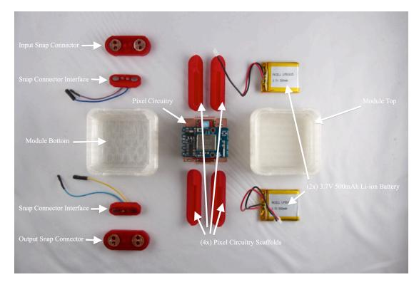
Figure 33: One complete Pixel module, opened and arranged to show the contained printed circuit board and parts.
