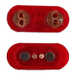
Figure 35: The front (top) and back (bottom) of the "snap" connection interface.
