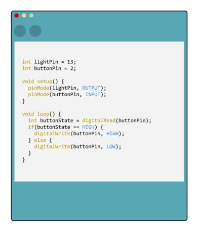
Figure 50: Drawing of the Arduino program for the light switch in Example 1, Part 1. This corresponds to Figure 6.
