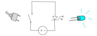
Figure 44: Conceptual drawing of the default "switch" behavior of a module represented as a switch circuit.
