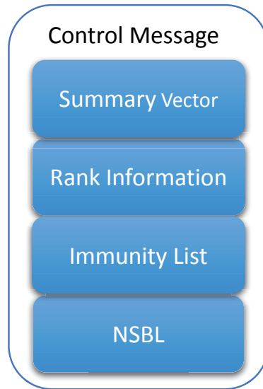
Figure 3.2: Structure of Control Message with Nullspace Stopping Condition
