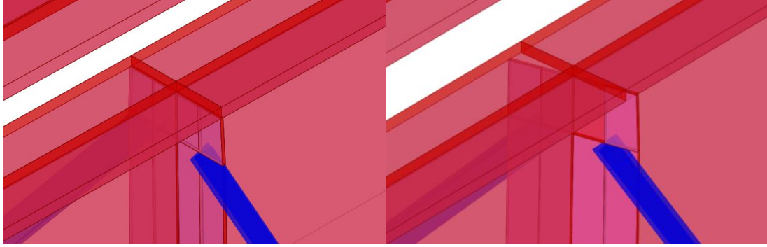
Figure 5.25 Skew (right) and non-skew (left) connection plates
