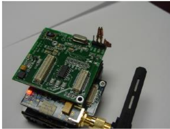
Figure 5.13 Wireless Sensor Imote2 (Measuring Acceleration and Temperature)
